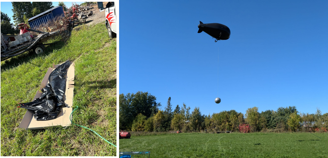
Figure 5.15: Left: blimp’s envelope being inflated with helium. Right: blimp with slung payload in neutral buoyancy.
