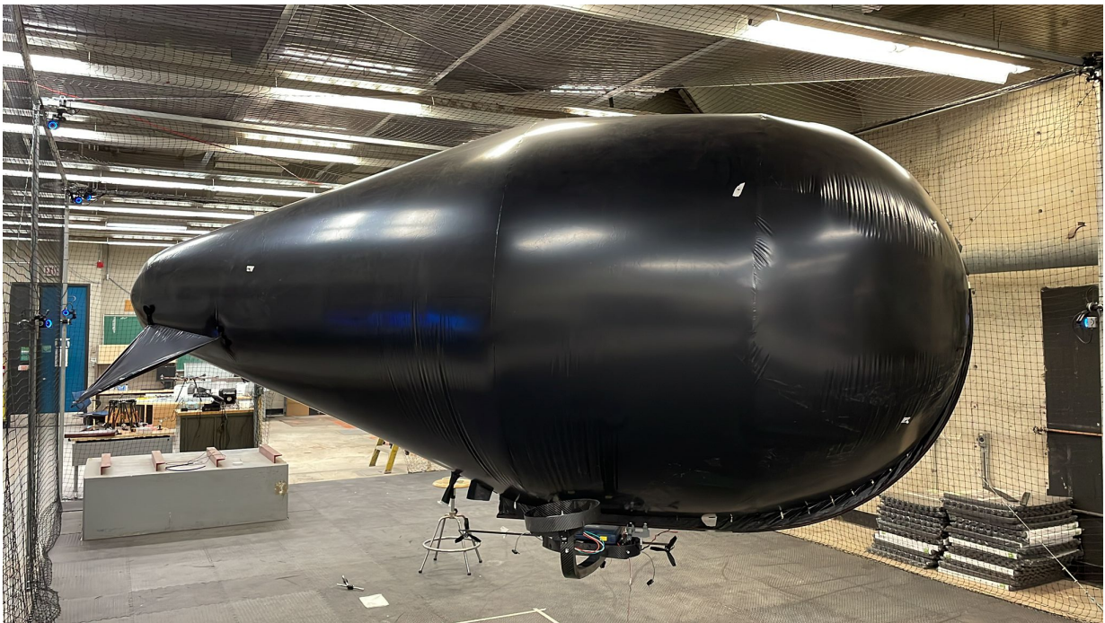
Figure 3.1: Physical prototype inside the experiment workspace. The cameras, emitting blue light, are used to capture the motion of the multi-body.
