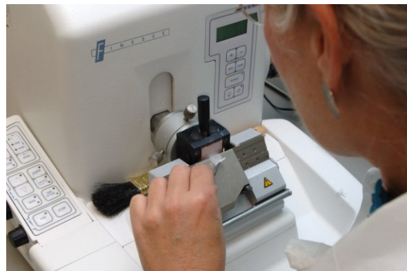
Figure 4 Block being sliced before staining and slide production 4
