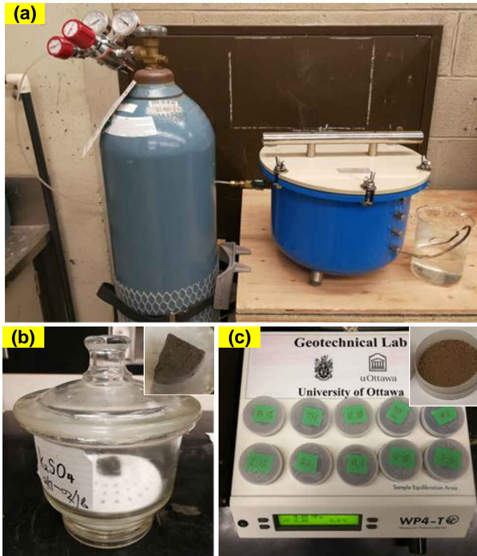
Figure 4.6 Three methods used for SWCC measurement: (a) Pressure plate method, (b) Vapor equilibrium method and cut saturated specimen, and (c) WP4-T measurement and wet soil aggregates
