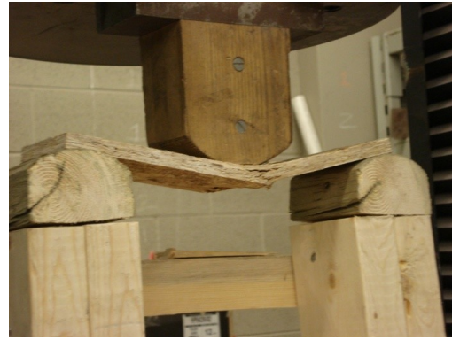
(b) Typical failure of sheathing coupons
