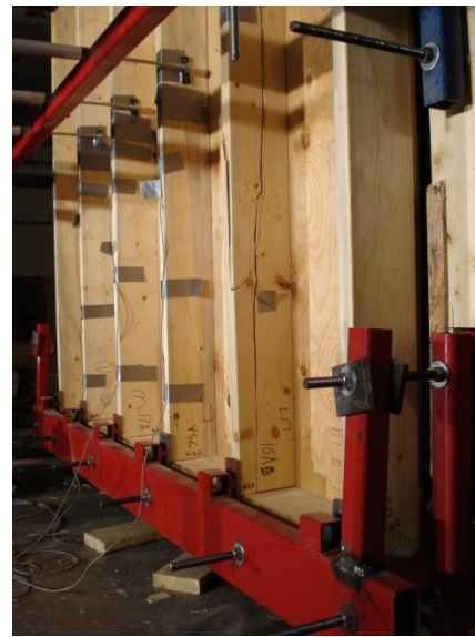
(c) Localize damage stud 5-Lower half
