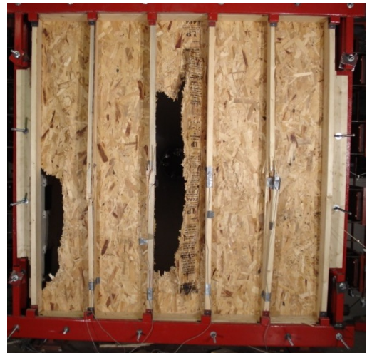
(b) View of sheathing failure
