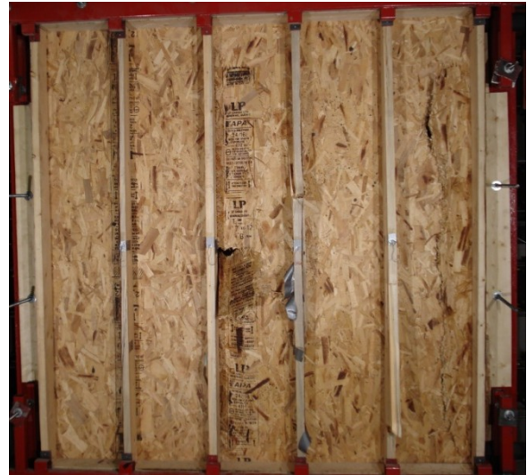
(b) View of sheathing failure
