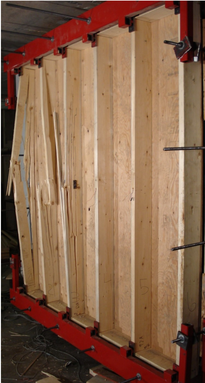
(b) Localized damage stud 1 to 3-Upper half
