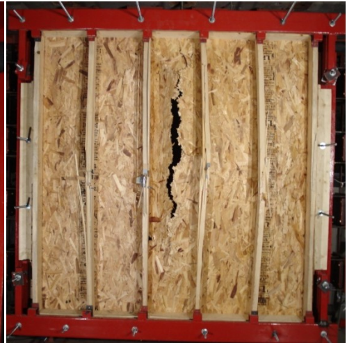
(b) View of sheathing failure
