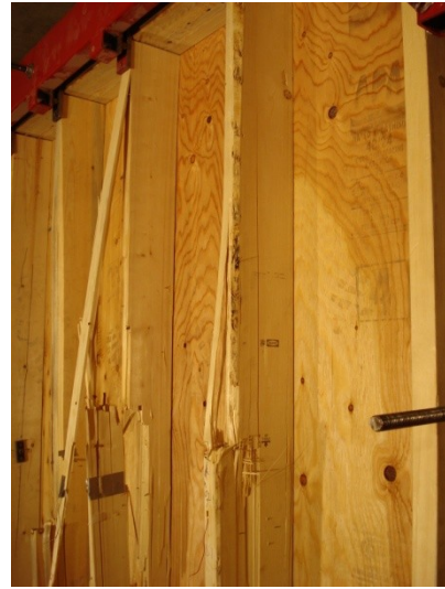
(b) Localized damage stud 1 to 5-Upper half
