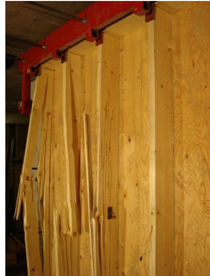
(b) Localized damage stud 1 to 3-Upper half
