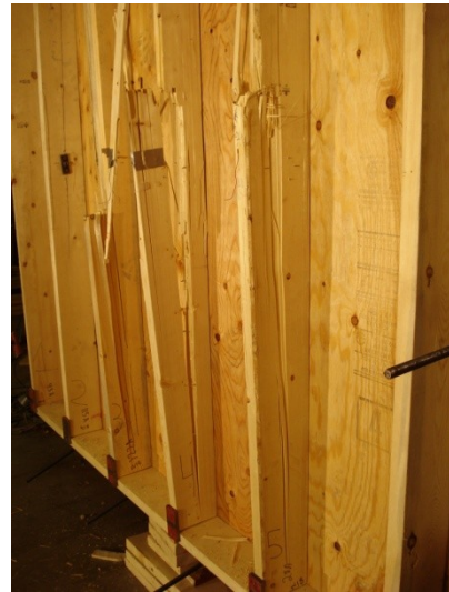
(b) Localized damage stud 1 to 5-Upper half
