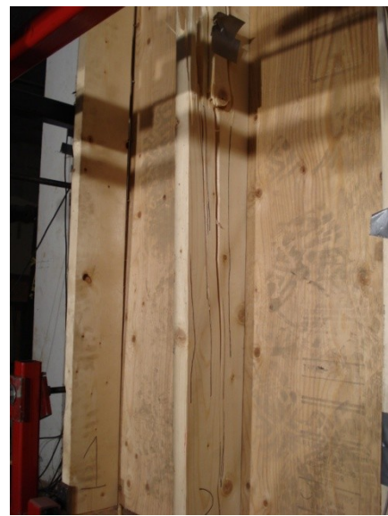
(c) Localize damage stud 2-Lower half
