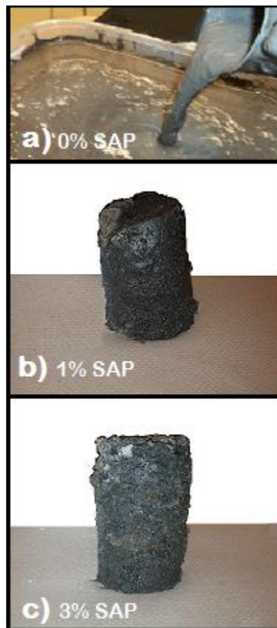
Fig. 3.6 Effect of changes made with direct method on the MFT with the addition of different amounts of SAP: a) 0%; b)1%; c) 3%
