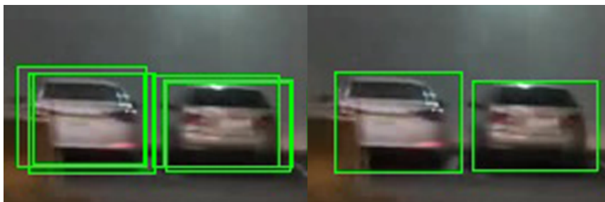
FIGURE 2.9: Prediction results before and after NMS. Left: before . Right: after.
