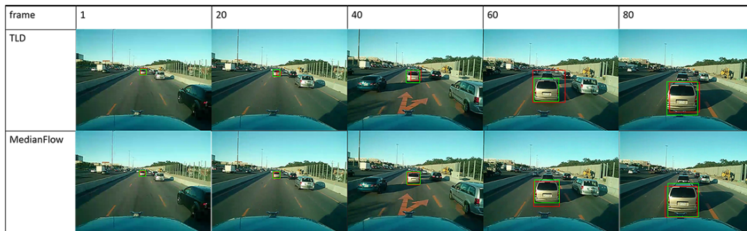
FIGURE 6.4: Tracking Result of the TLD and MedianFlow on Leading Vehicle.
