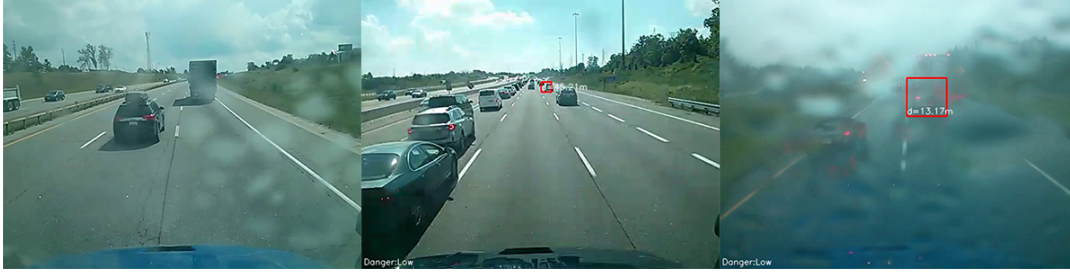
FIGURE 7.11: Failure cases of our FCW system in Python environment.
