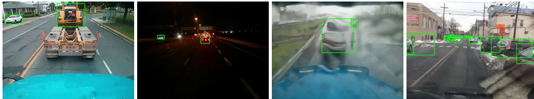
FIGURE 5.3: Failure cases of our SSD-LW-KM model.
