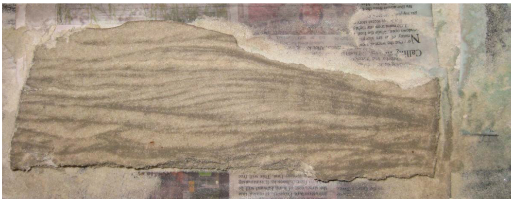
Fig. 3. Peel after applying dilute India ink.
