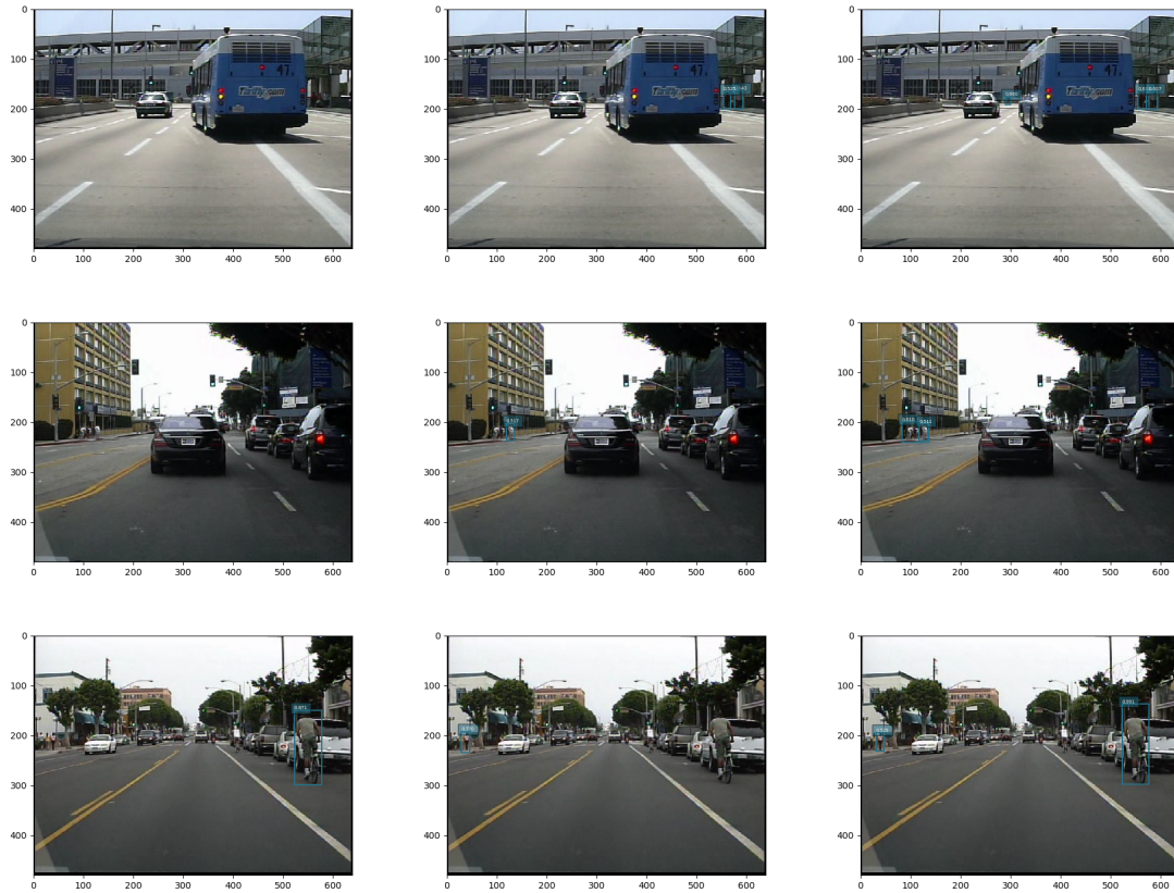
Figure 4.4: Demo on Caltech Pedestrian from SSD(left), SSD Customized(middle) and SSD Two-Stream(right). We can see that the original SSD and SSD Customized are good at detecting large and small objects respectively, while SSD Two-Stream takes advantages of both.
