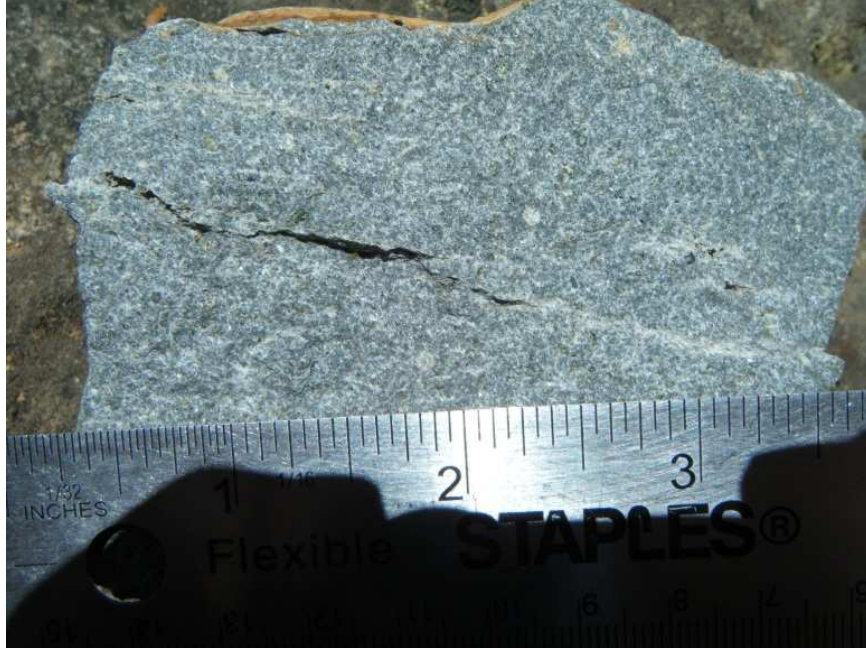
Plate 8: Tb 10LT-01. Olivine basalt with flow banding and foliated vugs.
