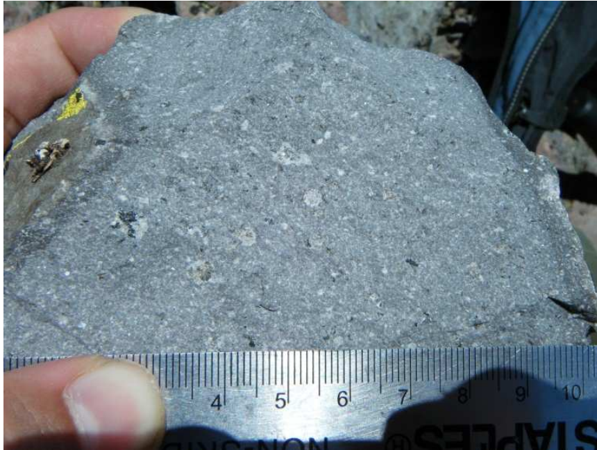
Plate 6: Tha 10LT-10. 2-4 mm phenocrysts of plagioclase and hornblende.
