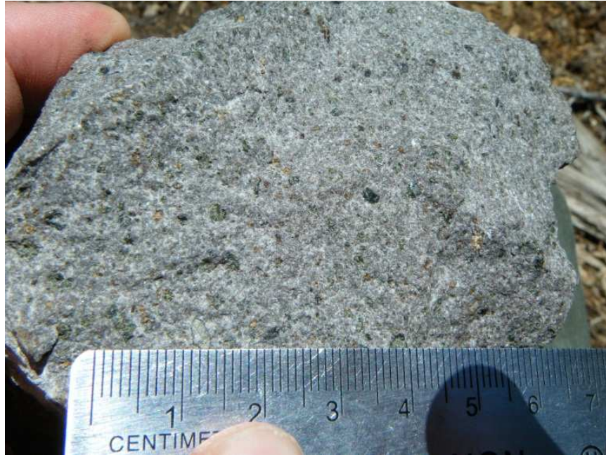
Plate 4: Tpap 10LT-03. 2-3 mm sized phenocrysts of pyroxene that are green, brown and black.
