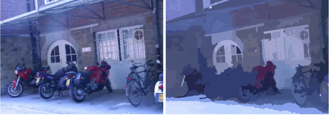
Figure 3.6: In comparison to the deviation and Chauvenet based outlier detectors the Q Test criterion is very restrictive. In this example of the bikes1 image from the experimental dataset only 147 segments were classified as potentially descriptive. The other two outlier detectors find more descriptive segments on the same example as shown in Figure 3.4 and Figure 3.5. Visually this difference can be seen by comparing the rightmost image of the three figures.
