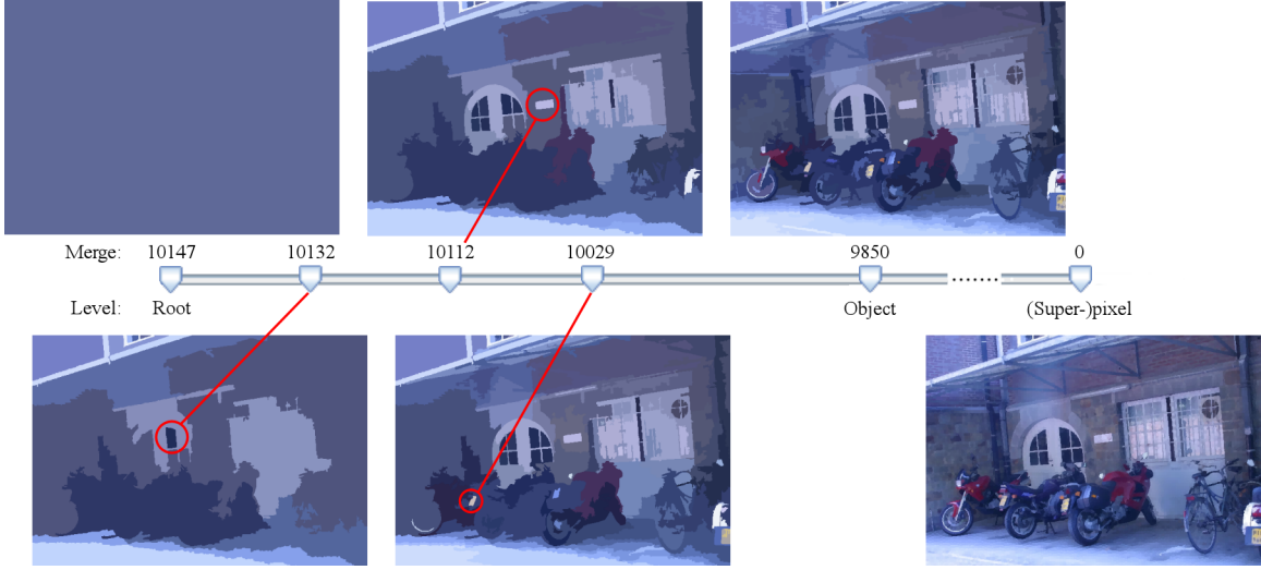
Figure 3.10: We browse through the merge history to find descriptive segments. Starting from the last merge (root level) we proceed until we reached the object level of the segmentation. We consider it unnecessary to go further than this object level because major segments were assembled at this point and mostly intermediate segments are merged before it. For every merge we compare the two segments involved to see if either of them complies with our definition of descriptive segments. In case one of them does, it is added to the set of descriptive segments. The example in this figure explains the process for the bikes1 image in our experimental dataset.
