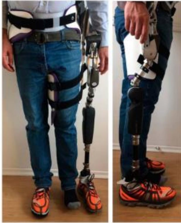
Figure 9-2 Hip disarticulation simulator setup with Helix 3D hip joint, showing 4 cm ground clearance on the prosthetic-side healthy limb [82]
