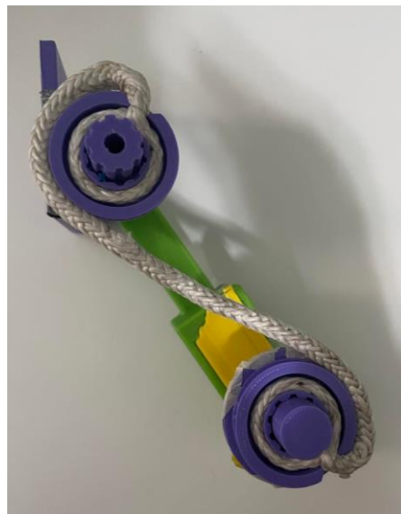
Figure 4-10 3D printed prototype of the rope and pulley design showing how the rope is anchored to the pulleys using loops on the ends
