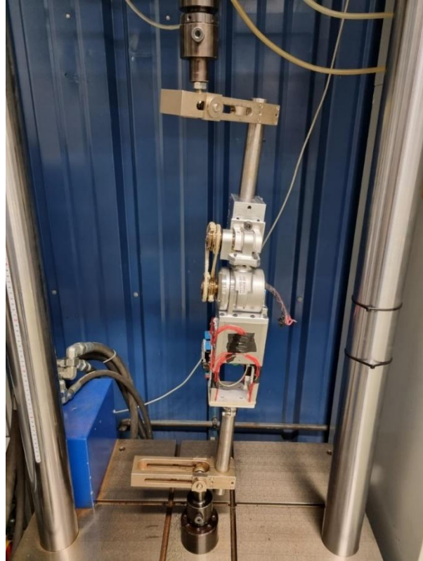
Figure 8-3 PHP in the testing machine for the M-L mechanical testing
