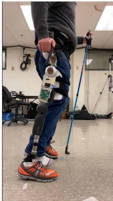
Figure 9-3 Hip disarticulation simulator with PHP, Össur Rheo 3 knee joint, and Össur Pro-Flex XC foot
