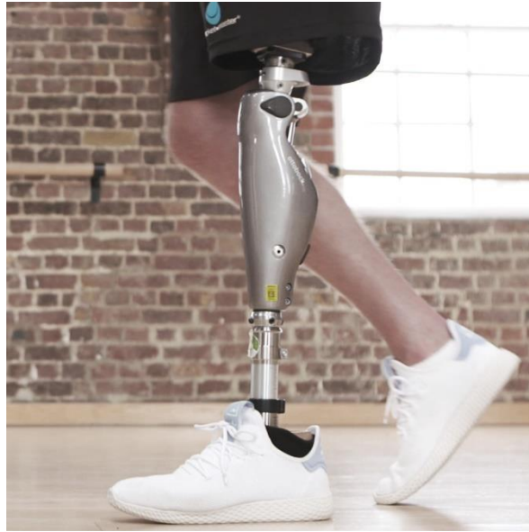
Figure 2-2 Ottobock C-Leg with microprocessor-controlled damping [11]
