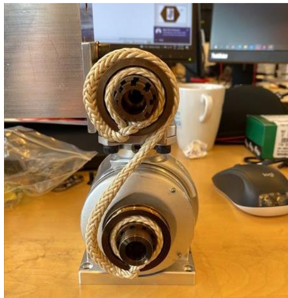
Figure 5-6 PHP ropes have loops that are anchored around the axle. The ropes exit through a hole in the pulley then wrap around the pulleys.
