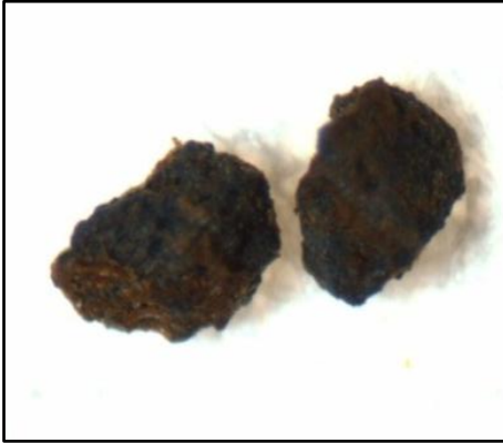
Figure A-2: Ferric iron hydroxide precipitates on the surface of GAC particles (mesh size 40×50) used in the isotherm experiment of ferric iron
