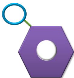
Figure 1.6: Schematic representation of helicase-avidin fusion protein. Helicase (purple) is fused with avidin (blue) by means of a short sequence of amino acids as a linker region (green).
