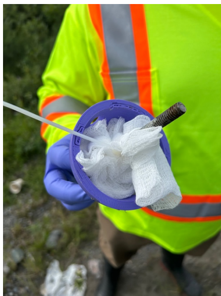
Figure 2.8. 3D printed COSCa passive sampler with sterile gauze.
