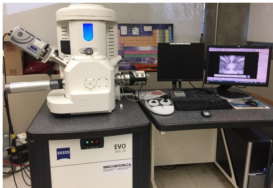
Figure A.10 Scanning electron microscope (SEM) (EVO-MA10, Zeiss, Germany) equipped with energy-dispersive X-ray spectrometer (EDS) (INCA-x-act, Oxford Instruments, UK) for microstructure and chemical composition characterization
