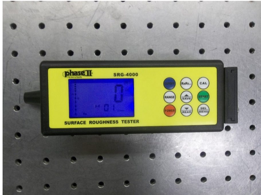
Figure A.6 Stylus surface roughness tester (SRG-4000, Phase II Plus, USA)
