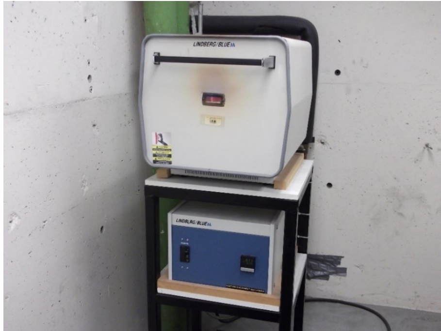
Figure A.2 Laboratory furnace (Lindberg/Blue M™, Thermo Scientific™) for superalloy heat treatments and isothermal oxidation evaluation
