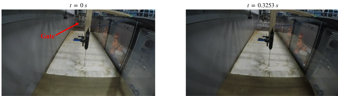
Figure 3.3: Snapshots of gate opening at t=0 s (left) and t=0.3253 s (right) for the test SC-H1
