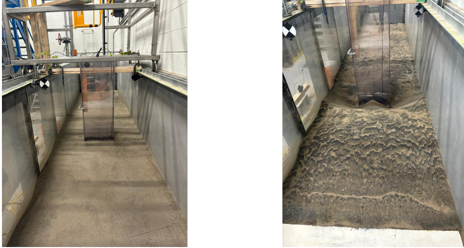
Figure 5.2: Snapshots of the sediment section (a) before and (b) after the test
