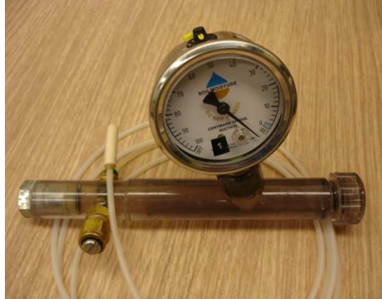
Figure 3.7 : Tensiometer with a vacuum gauge and other accessories
