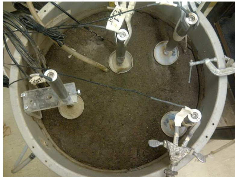
Second Preliminary test showing LVDT's used for surface deformation on Loam soil
