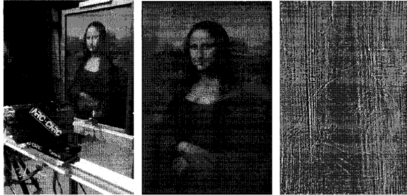
Figure 5: Images from the NRC's 3D Exploration of the Mona Lisa Project [4]. Left to right: The portrait being scanned by the NRC high-resolution color laser scanner; the scanned image; and a depth image of the Mona Lisa showing the surface's texture.
