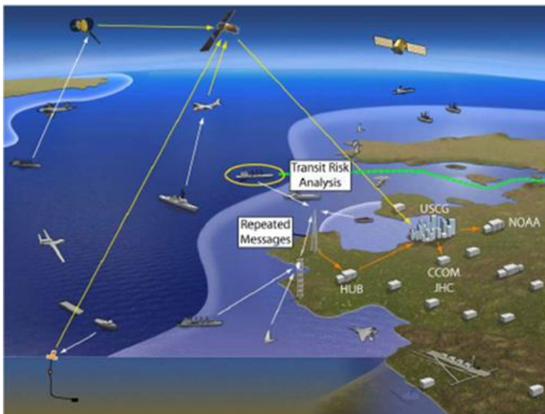
Figure 2.2: Schematic view from the United States Coast Guard of how AIS messages are transmitted and received from vessel to vessel/satellite or terrestrial receiver (from Calder et al., 2009).
