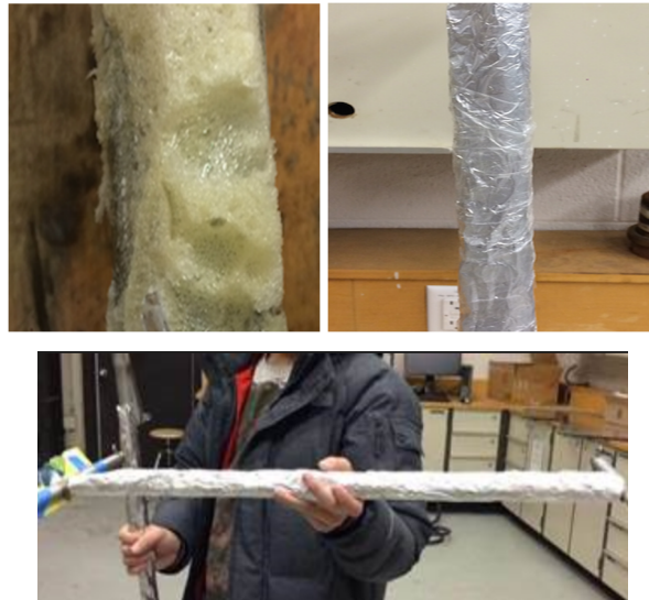
Figure 3.5 The bridge cable model with 2.0 cm ice accretion a) initial foam model b) improved model
