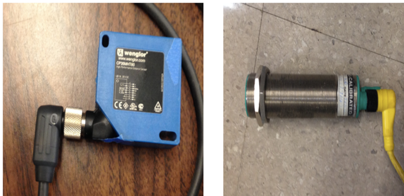
Figure 3.29 The displacement sensors used in the wind tunnel
