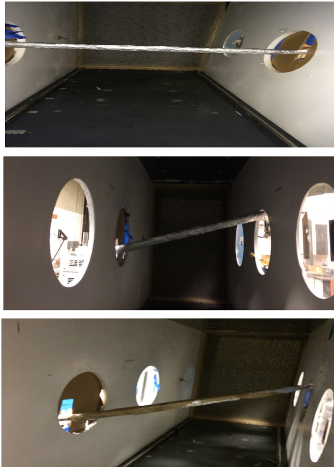
Figure 3.6 The cable models in wind tunnel a) Model 1, case \alpha = 0^\circ , \beta = 0^\circ b) Model 2, case \alpha = 0^\circ , \beta = 15^\circ c) Model 3, case \alpha = 30^\circ , \beta = 15^\circ
