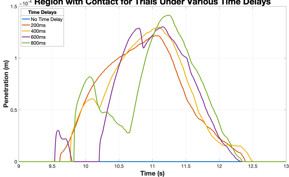
Figure 59: Region Between 9-13 Seconds for the Penetration Depth of Trials from Experiment 3, Scenario 2 that are Subjected to Various Time Delays.
