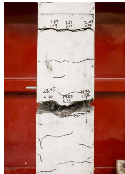
g) Mid-span fibre pulled out at Blast 4
