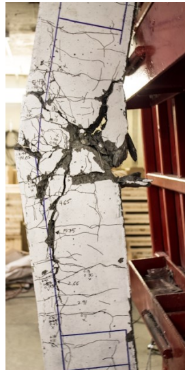
d) Mid-span crushing & fibre pulled out at Blast 5, HSC-F0.5(5D)-20M-S
