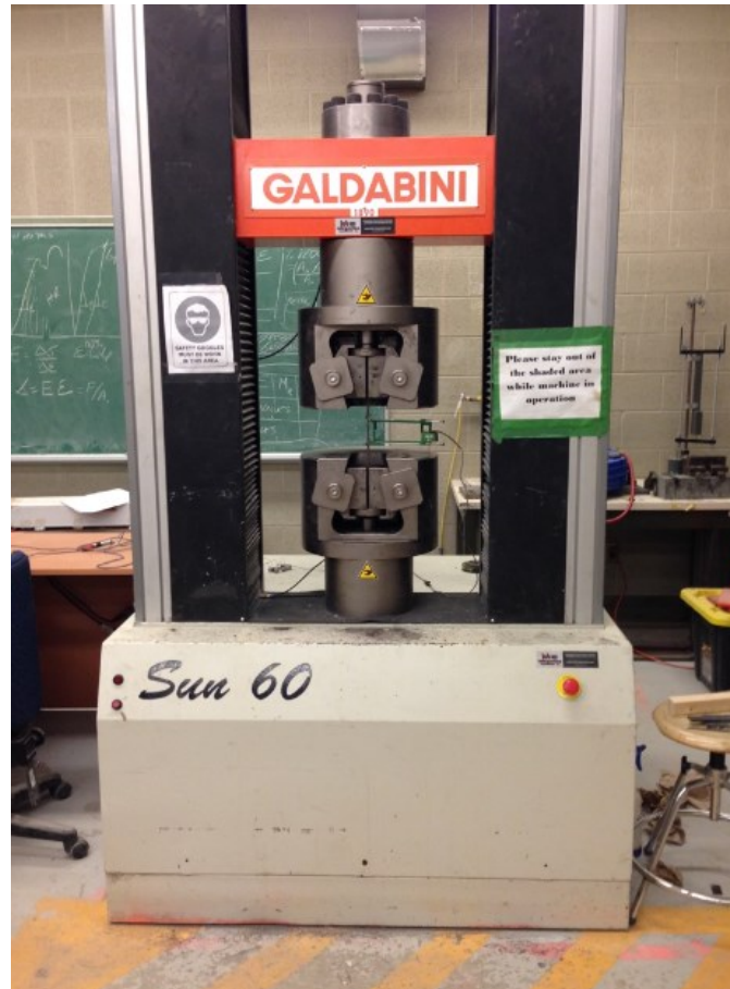
Figure 3-4 GALDABINI Universal Floor Standing Testing Machine and Axial Extensometer; testing steel rebar
