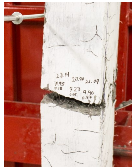
h) Mid-span fibre pulled out at Blast 5
