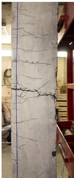
e) Mid-span cracking at Blast 3
