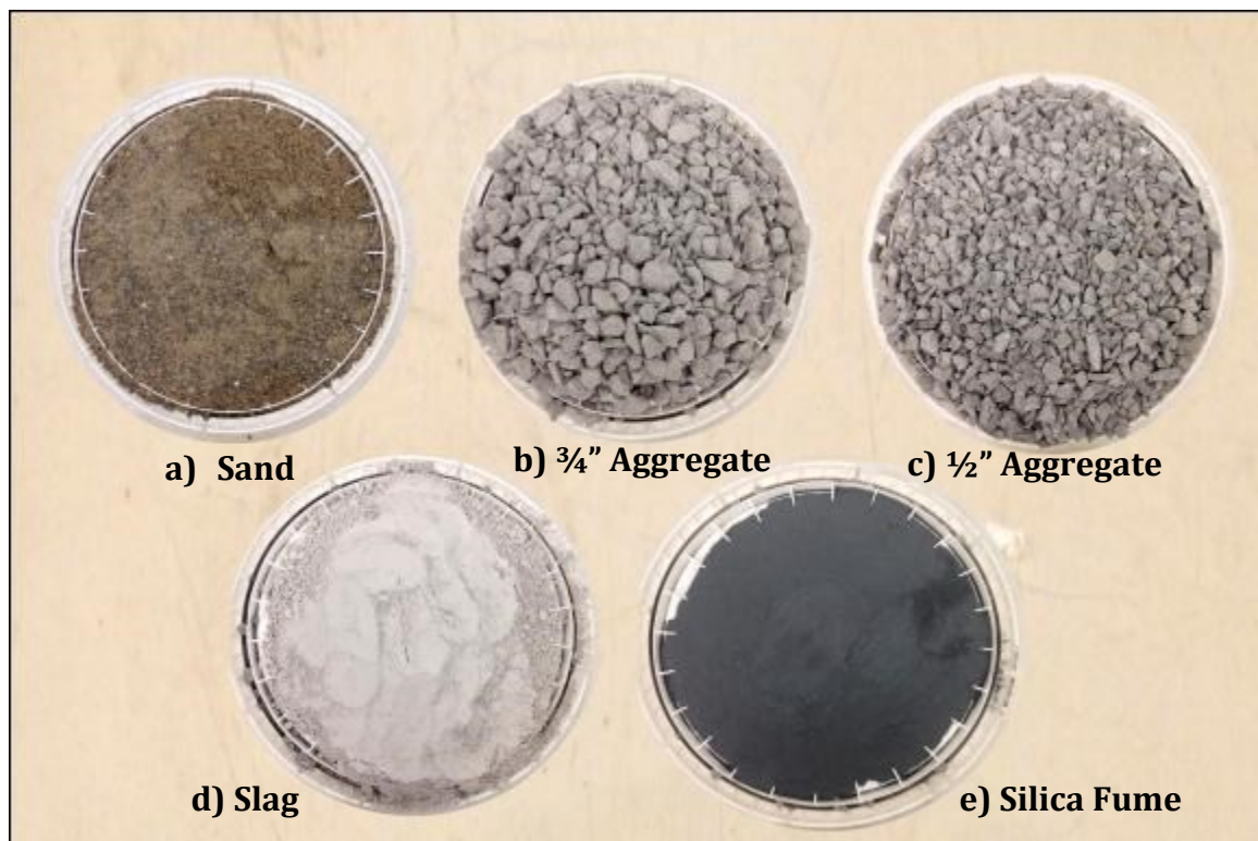
Figure 3-3 High strength concrete materials
