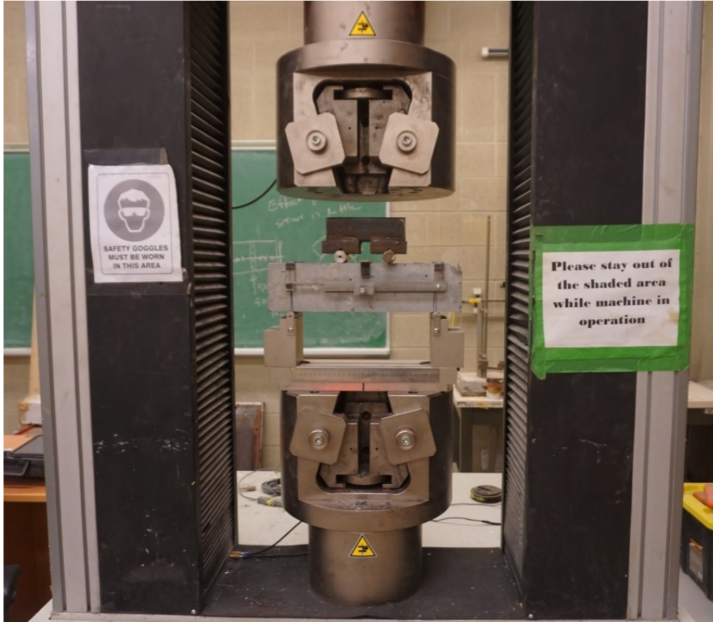
Figure 3-16 Flexural beam testing setup
