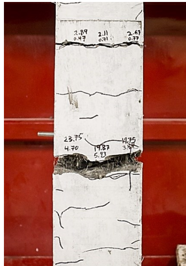
g) Mid-span fibre pulled out at Blast 4, HSC-F1(ZP)-15M-0
