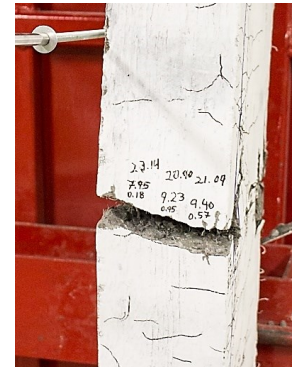
g) Mid-span fibre pulled out at Blast 5, HSC-F1(ZP)-20M-0
