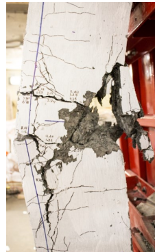
f) Mid-span crush & fibre pulled out at Blast 5, HSC-F1(ZP)-20M-S
