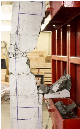
g) MID-span crushing at Blast 3, HSC-F0-15M-S
