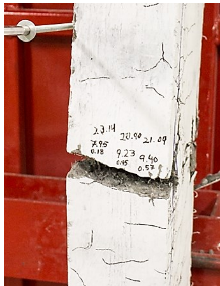
c) Mid-span fibre pulled out at Blast 5, HSC-F1(ZP)-20M-0
