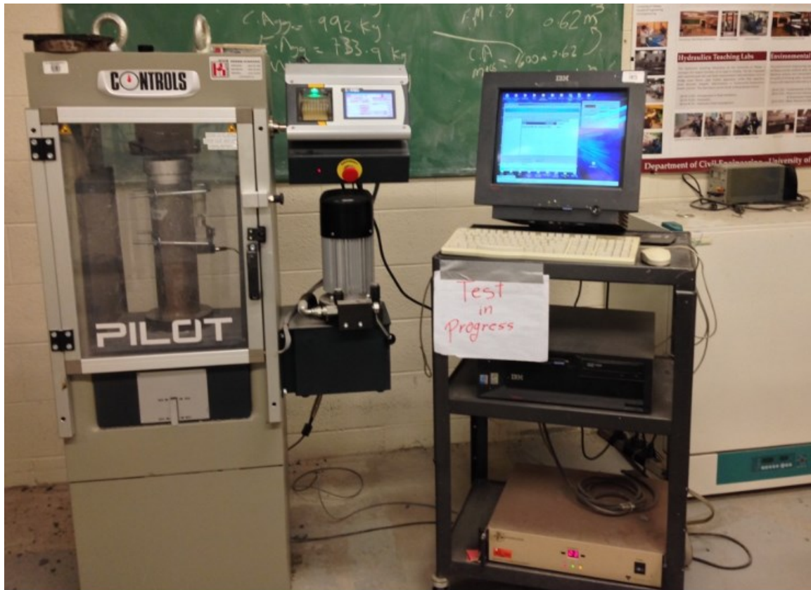
Figure 3-13 Cylinder testing setup
