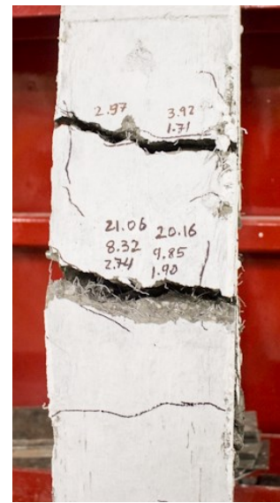
h) Mid-span fibre pulled out at Blast 5
