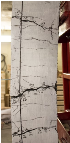
f) Mid-span cracking at Blast 3
