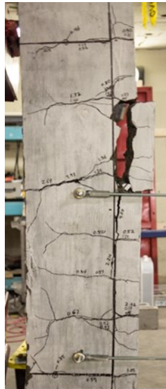
c) Mid-span spall at Blast 2A, NSC-F0-#4-S
