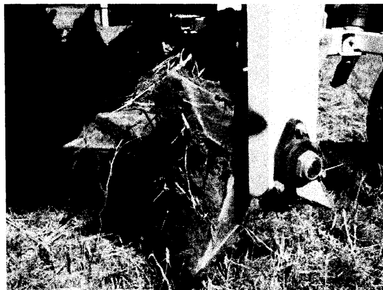
Figure 2.17 Clogging of the AerWay tine when running the implement on very wet soil.
