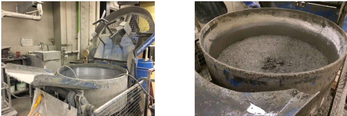
Figure 3-8 Concrete pan mixer used to cast all beams
