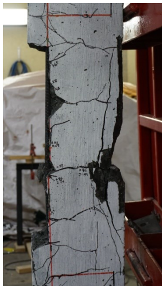
f) Mid-span cracking at Blast 3b
