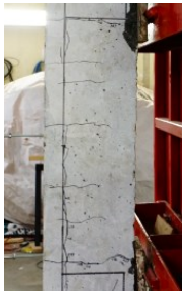
f) Mid-span cracking at Blast 3b
