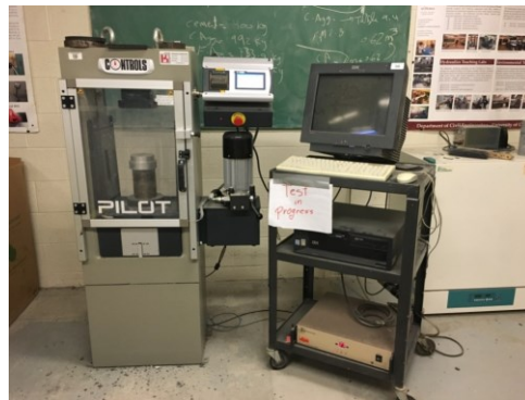
Figure 3-10 Cylinder testing setup
