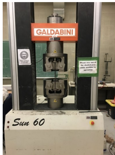
Figure 3-3 GALDABINI Universal Floor Standing Testing Machine; testing steel rebar
