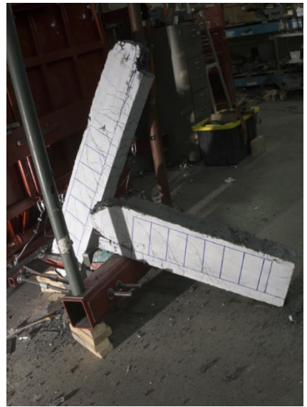
i) Tensile Reinforcement bar ruptured at blast 6
