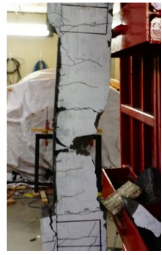
e) SCC-F0-#4-S Mid-span spalling at Blast 3b (50 psi)
