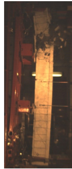
g) Secondary fragmentation during blast 4
