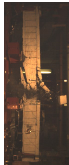
g) Concrete split out and secondary fragmentation during blast 4
