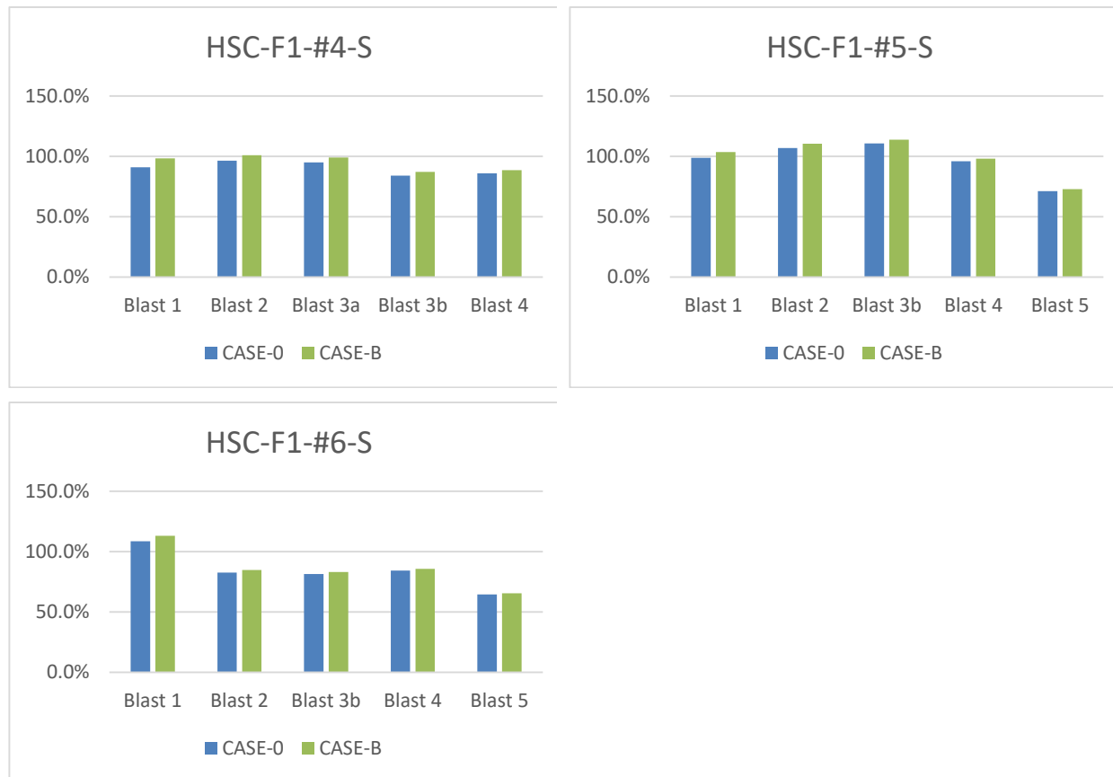
Figure 7-26 Sensitivity analysis for HSFRC specimens – DIF for concrete in tension
