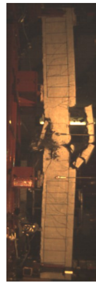
g) Concrete split out and secondary fragmentation during blast 3b
