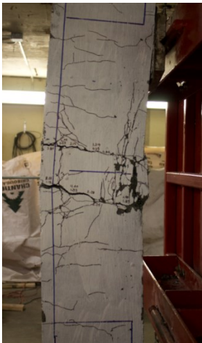
c) HSC-F1-20M-S-400 Mid-span damage at Blast 4 (70 psi)
