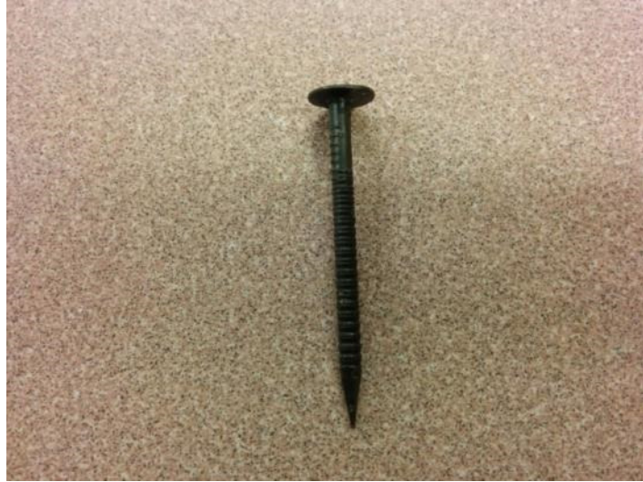
b) 12.5 Gauge GWB Nail Picture
