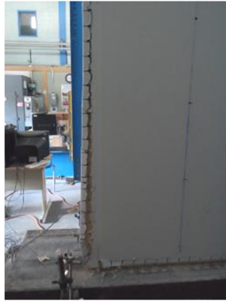
a) Wall 8-2 GWB Fissure Failure Mode
