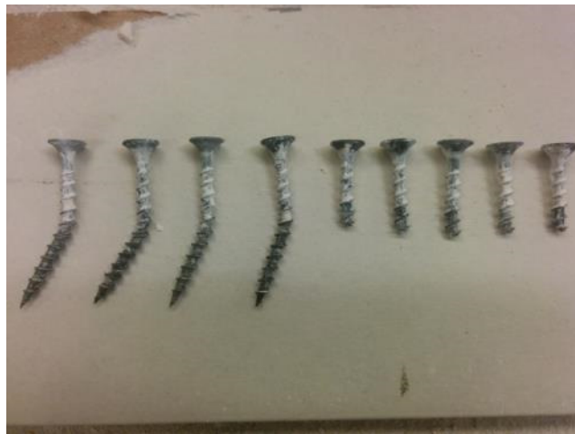
Figure 23: Bent and Ruptured Screws
