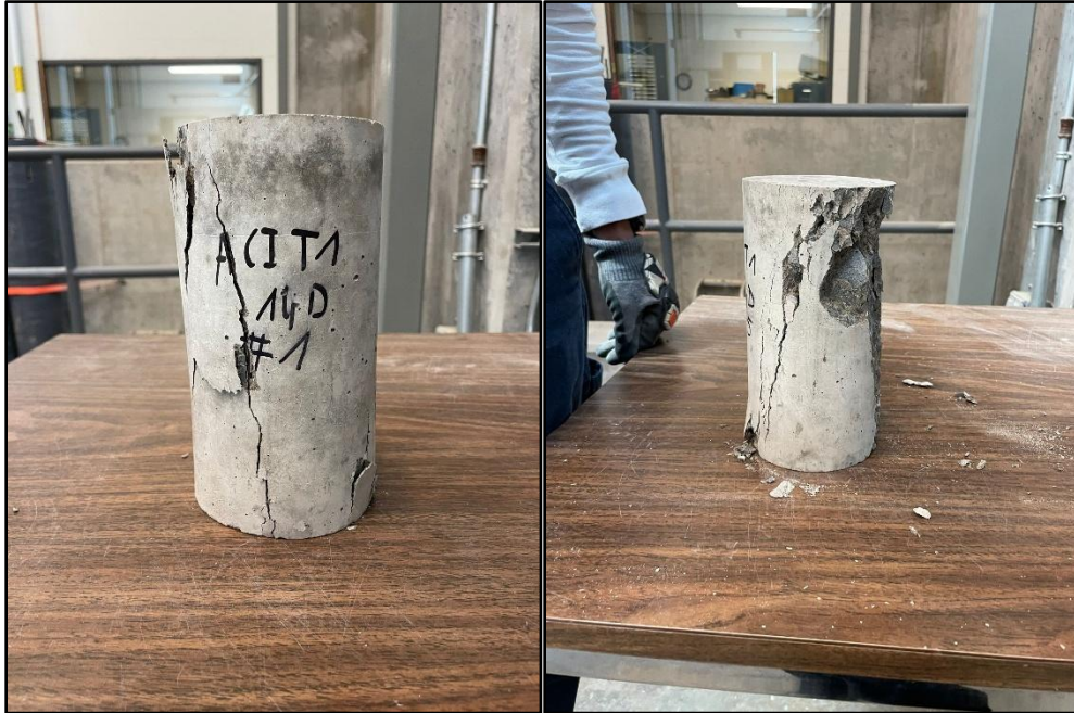
Figure 3-39: Failure mode prior to compression machine lubrication.
