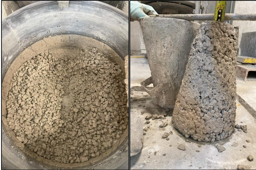
Figure 3-29: EMVc-TB4-1 fresh state.
