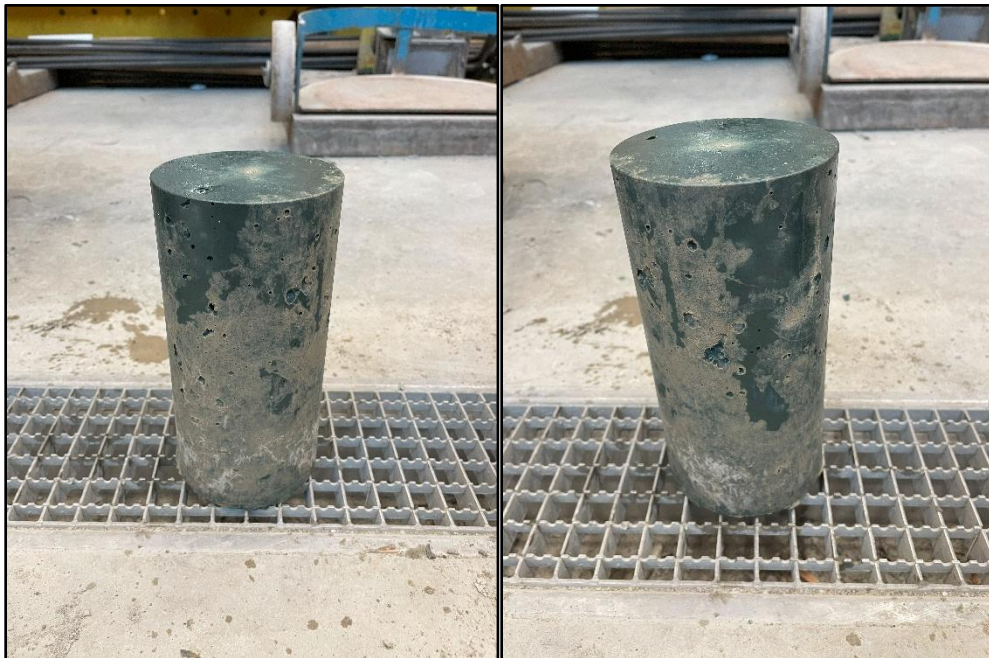
Figure 3-30: EMVc-TB4-1 demoulded cylinder.
