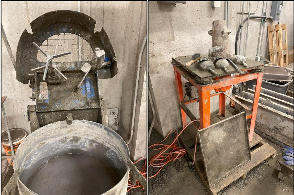
Figure 3-10: 60L pan mixer and accessories.
