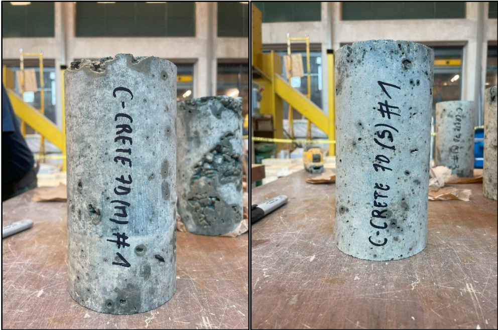
Figure 3-31: EMVc-TB4-1 moist- and submerged-cured cylinders.
