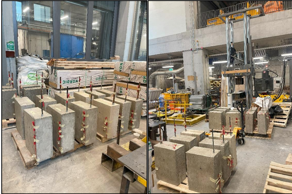
Figure 4-26: Beam-ends placing in the testing area.
