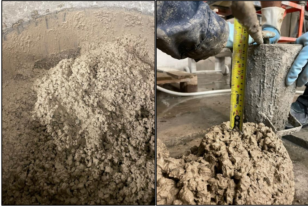
Figure 3-37: EMVc-FM-1 fresh state.
