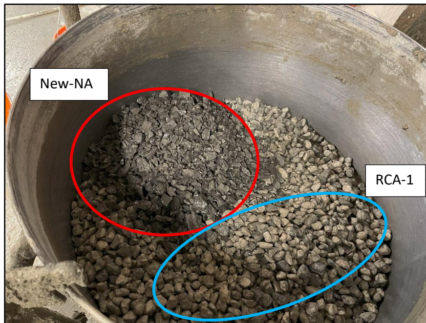
Figure 3-9: Visual comparison between natural coarse aggregate and RCA.
