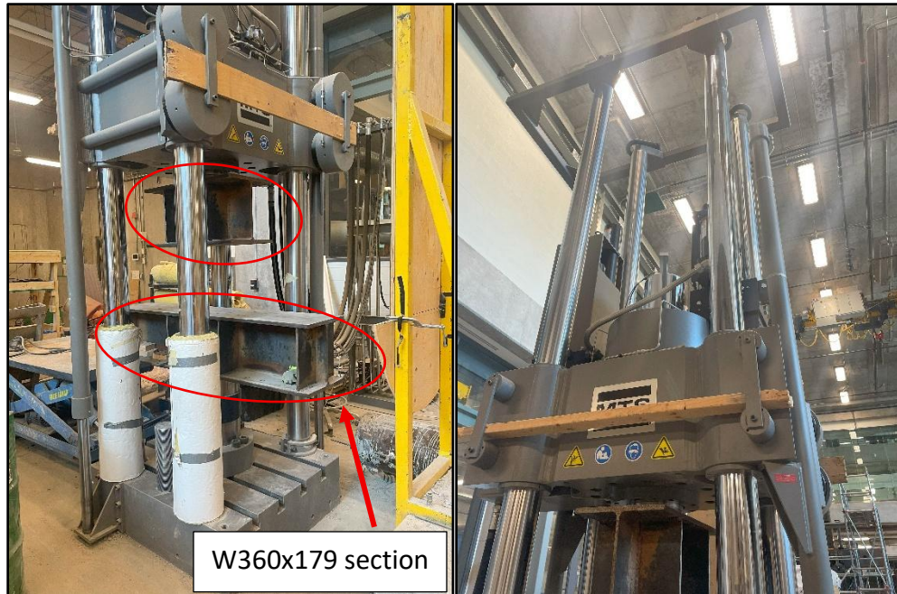
Figure 4-8: MTS 311.51 High-Force Test System.
