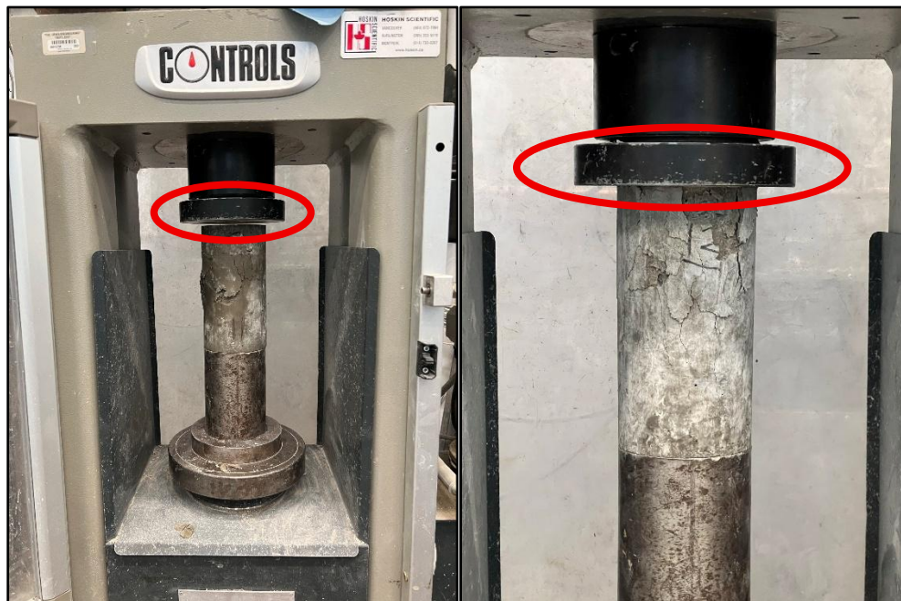
Figure 3-38: Automatic concrete compression machine.
