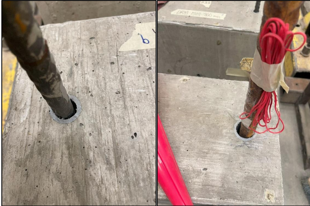
Figure 4-91: Clearance between PVC bond breakers and reinforcement.
