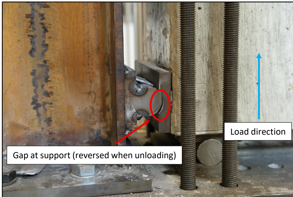
Figure 4-49: ACI-15M-170-C support movement during bar pulling.
