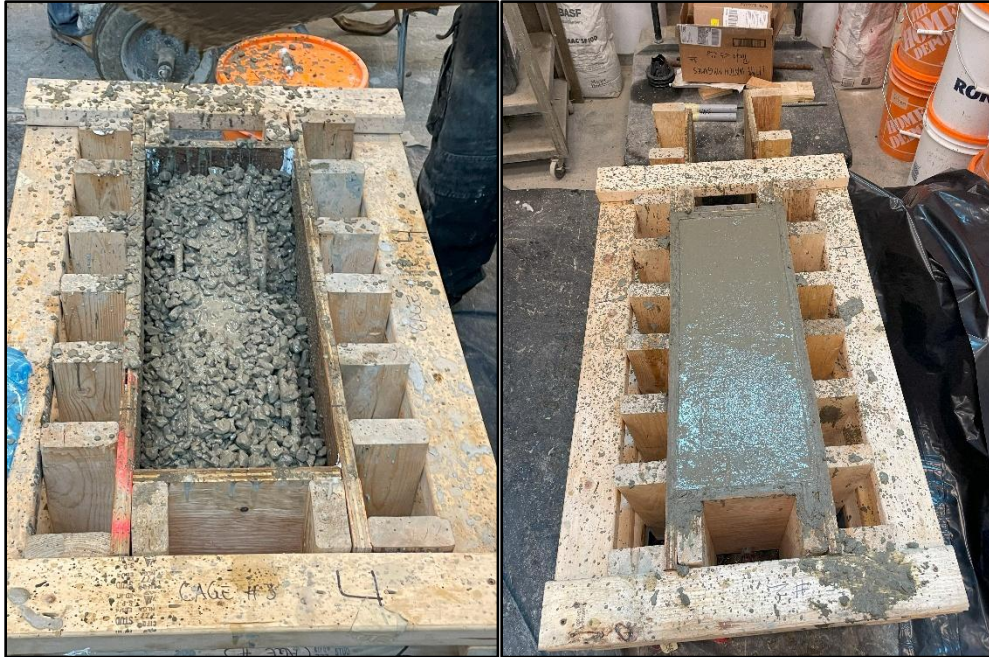
Figure 4-24: Beam-end casting and finishing.
