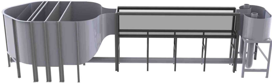
Figure A.1: A SolidWorks model of the new water tunnel facility; model created by myself and Rachel Andersen.
