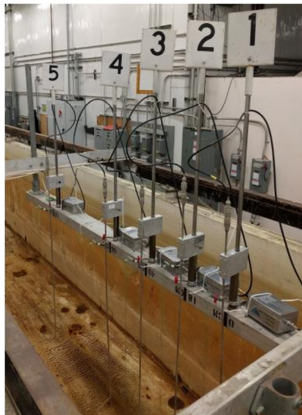
Figure 4-6: Five wave gauges' array and probe labeling
