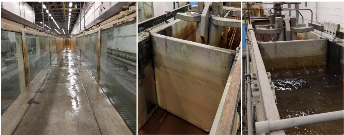
Figure 4-1: NRC-OCRE Steel Wave Flume (SWF) and wave generator.
