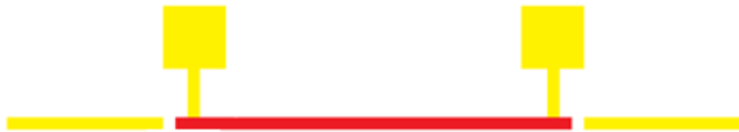
Fig. 1.4 Sketch of an LRSPP straight waveguide for thermo-optic modulation.
