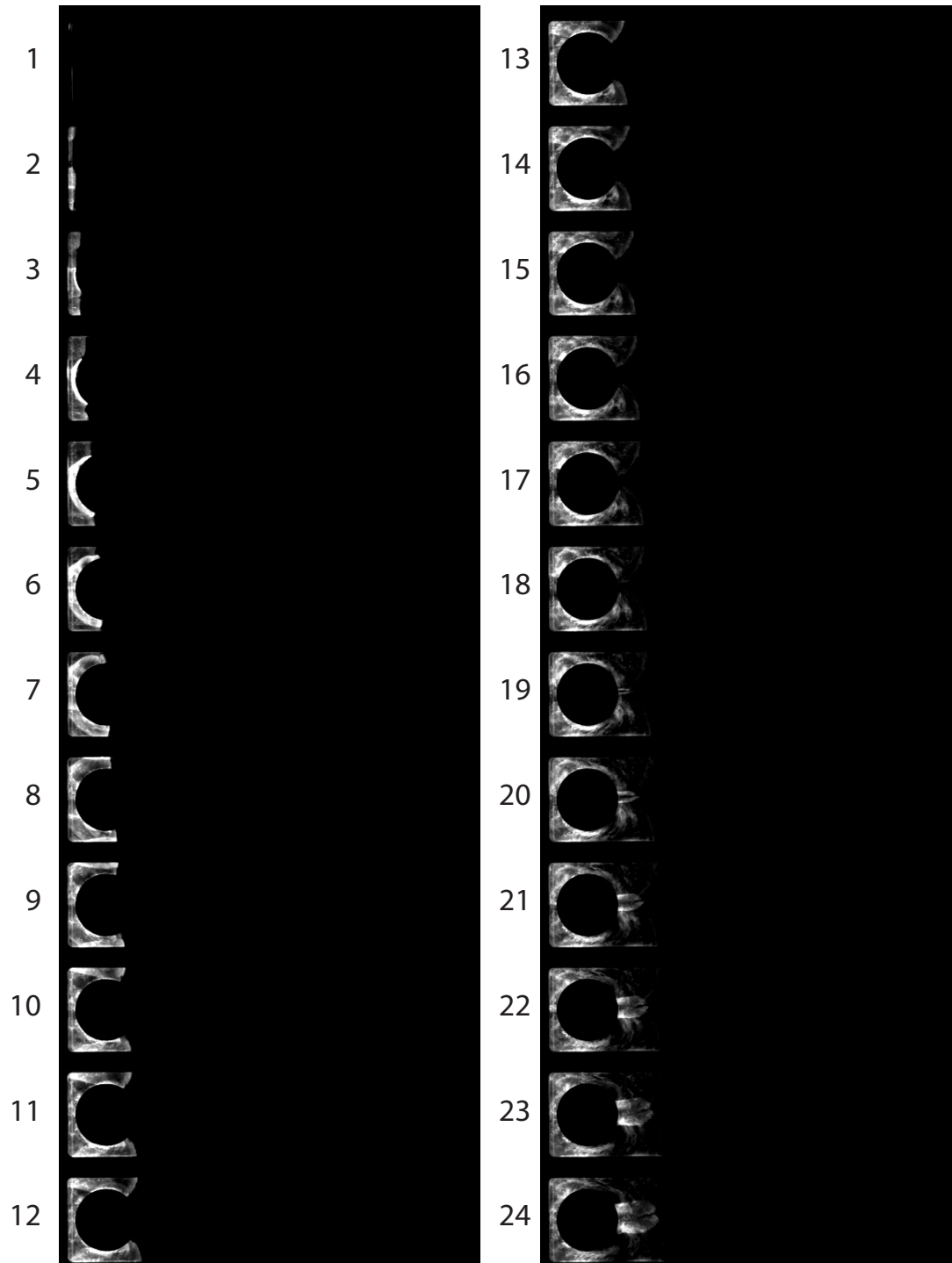
Figure F.21: Part 1 of Direct visualization record of the self luminosity in methane-oxygen at p_0 = 6.9 kPa
