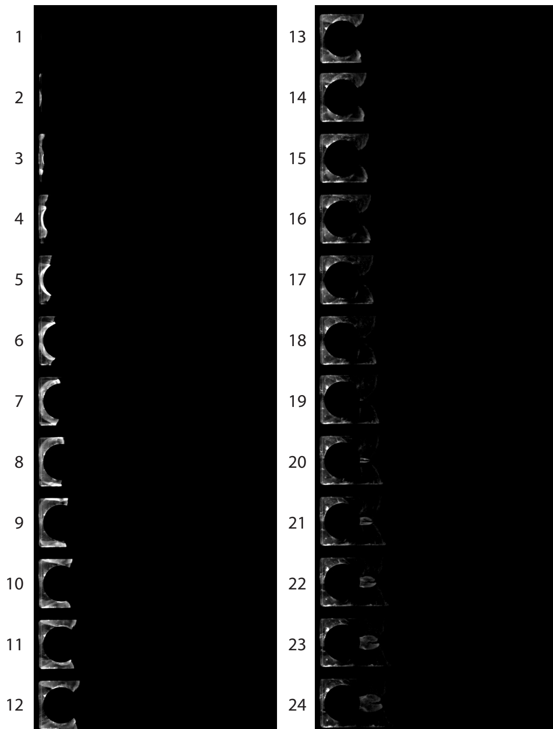
Figure F.25: Part 1 of Direct visualization record of the self luminosity in methane-oxygen at p_0 = 6.9 kPa
