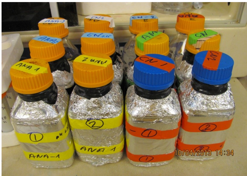
Figure A-8. The experimental microcosm bottles in the anaerobic chamber were protected from light by covering them with Al foil.
