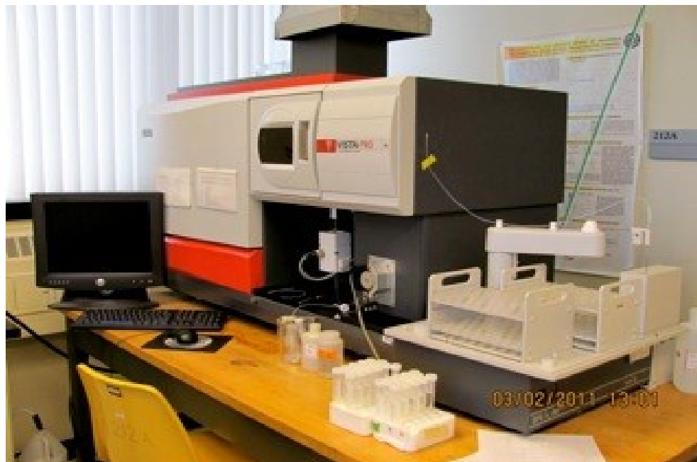
Figure A-5. Figure A-5. The analyses of the aqueous phase in this research were performed with the Varian Vista Pro ICP-OES instrument.
