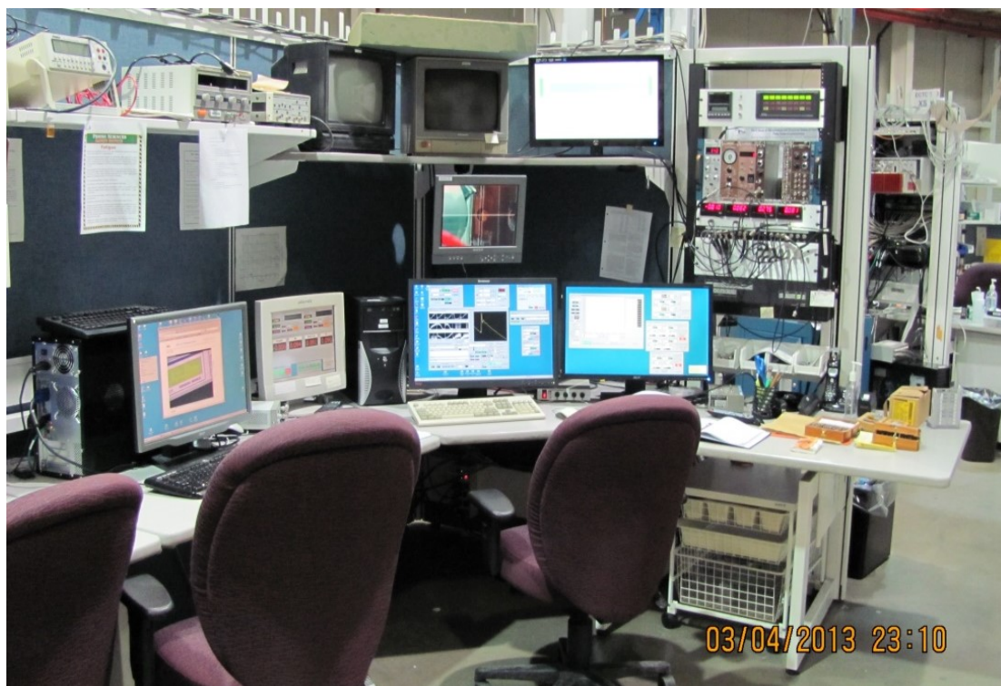
Figure A-10. The XAS control desk during data acquisition. The output parameters, such as the temperature, input-output energy and the XAS signal were monitored as shown on the computer screens from left to right.
