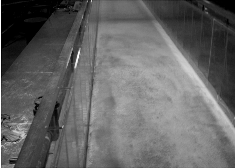
Figure 9.3 Condition of bed after fixed bed (FB) test run in large flume
