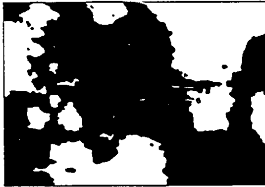
Fig. 3.4 Shore line of a simulated fractal surface having D_f = 2.2 . This is an example of statistically self-similar fractal. Instead of appearing exactly self-similar under magnification changes (as does the von Koch curve), this pattern has identical statistical properties over a range of scales. (Modified after Voss, 1988).
