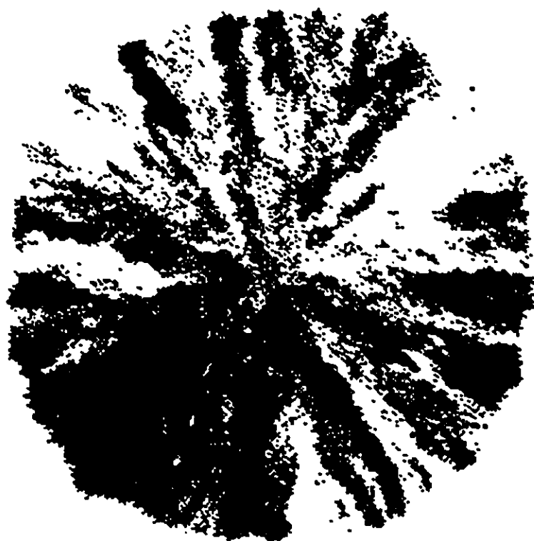
Fig. 5.13 Typical slit island section through computer generated plumose joint formed in medium containing 20% defects.
