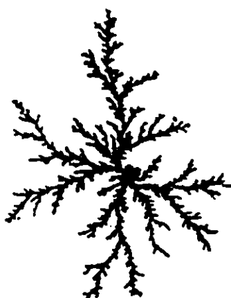
Fig. A.9 Image of fractal dissolution network from 2-dimensional radial dissolution experiment (after Daccord, 1987). Water was injected at center, and over time dissolution of the porous medium (plaster) resulted in the fractal pattern. Note the similarity with Fig. A.8. See text for more discussion.
