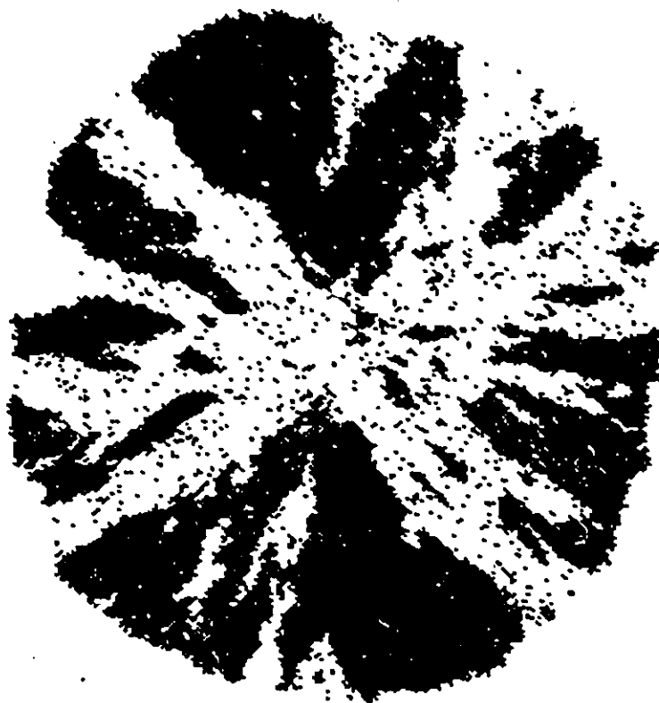
Fig. 5.10 Typical slit island section through computer generated plumose joint formed in medium containing 2% defects.
