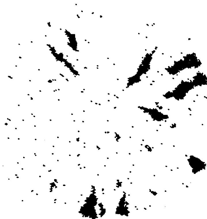
Fig. 5.7 Typical slit island section through computer generated plumose joint formed in medium containing 0.2% defects.
