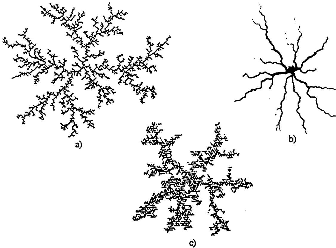
Fig. A.5 Similar fractal patterns formed by different physical process. a) Results from diffusion-limited aggregation (DLA) program, D_f=1.7 (see Appendix B). b) Dielectric discharge on a glass plate, D_f = 1.7 (Niemeyer et al. , 1984). c) Simulated uniform dilational fracture, D_f=1.55 (Louis and Guinea, 1987). All patterns demonstrate scale-invariant branching.
