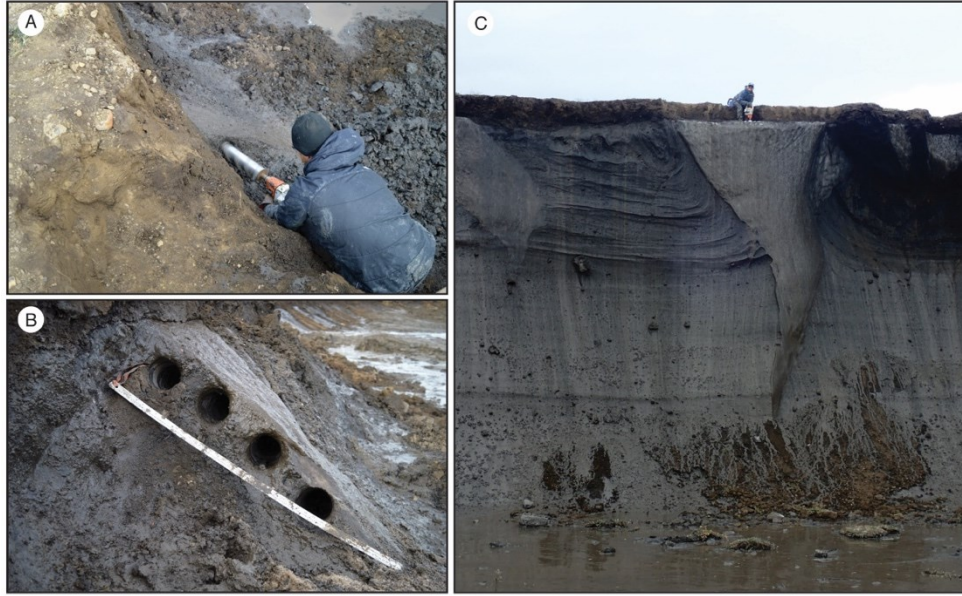
Figure 4.2. Images of ice wedge sampling. (A-B) horizontal drilling of ice wedge at Dump slump (EU18-W2), (C) vertical samplings of ice wedge at Mokka Fjord (MF-W3).
