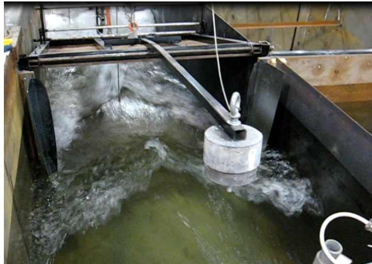
Figure 4.3: Formation of cross-waves upstream and downstream of the gate apparatus (Courtesy of Taofiq Al-Faesly)
