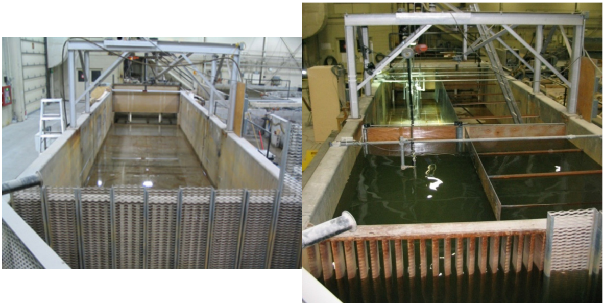
Figure 4.1: The High-Discharge Flume before (a) and after (b) modification for the testing program (Courtesy of NRC-OCRE and Taofiq Al-Faesly)
