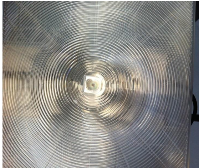
Figure 5-12: Individual optic 4 – no evidence of any abnormalities
