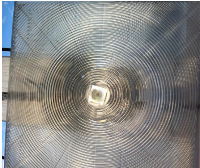
Figure 5-18: Individual optic 7 – no evidence of any abnormalities.
