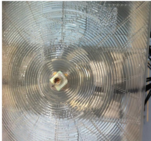
Figure 5-10: Individual optic 3 – significant water ingress and charring of the reflector.
