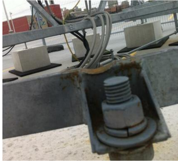
Figure 4-9: Divot formed in tracker rail due to the grinding of the drive wheel on the tracker ring.
