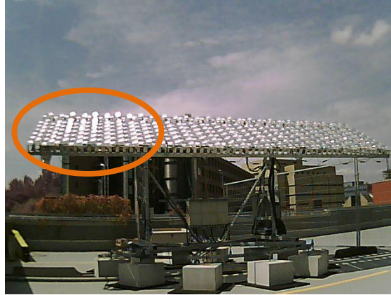
Figure 4-5: Tracker 1 tracking only in elevation. Glare, or reflections off of the left side of the tracker makes it apparent the tracker is not on-sun.
