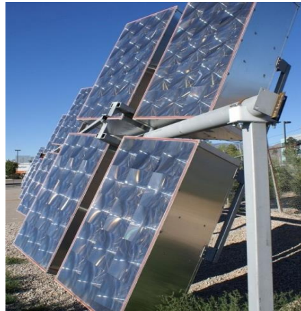
Figure 2-9: Suncore CPV panel on tilt and roll tracker.
