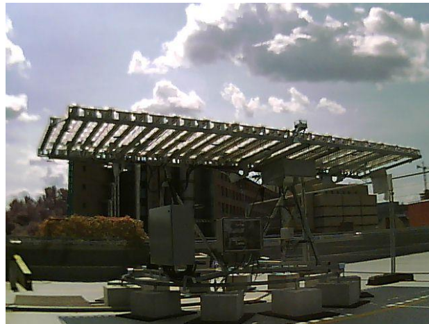
Figure 4-6: Tracker 1 tracking only in azimuth. Elevation position of tracker remains stow.
