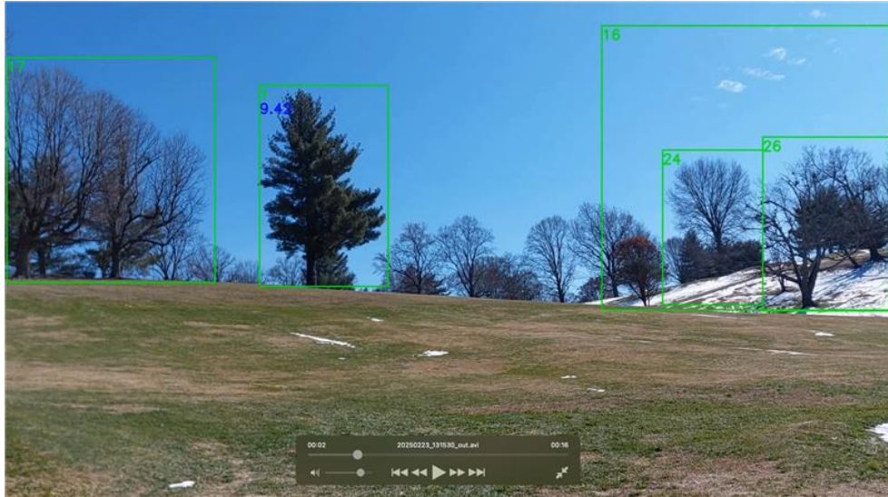
Figure 5.7: YOLOv8 detects tree crowns (green boxes) in a Phase 2 frame. Numbers indicate detection confidence scores.
