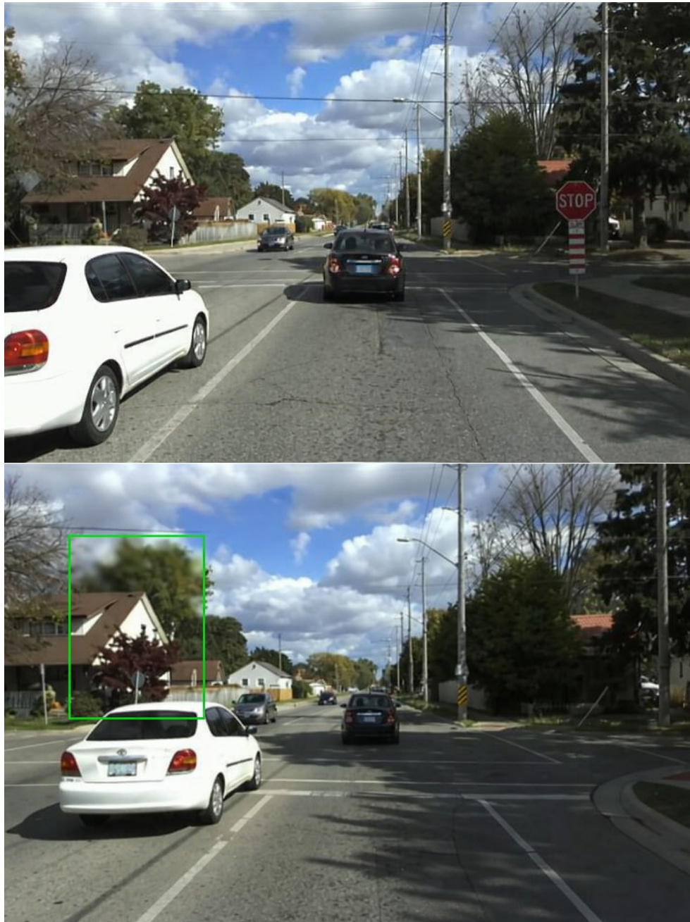
Figure 4.7: Phase 2 detection example. Top: raw frame from the vehicle-mounted camera. Bottom: the same frame after YOLOv8 tree detection, showing the bounding box and predicted wind speed overlay.
