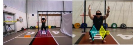
Fig 1. Visual representation of the recorded 2D video (60-Hz frame rate) and hip-knee-ankle angle measurements of OHS movement being analyzed using Kinovea software.
