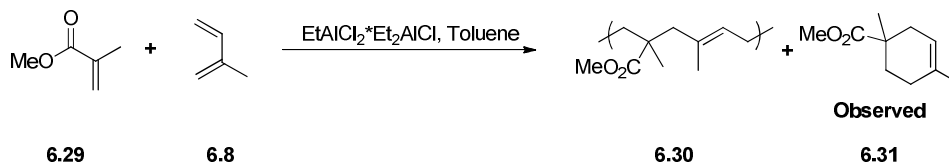
Scheme 55: Diels-Alder adduct observed during co-polymerizations when EASC is used as catalyst
