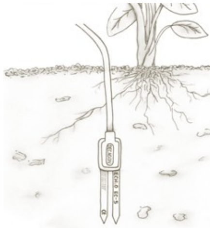
Figure G-1 Installation of the EC-5 sensor (Courtesy of Decagon, Inc.)
