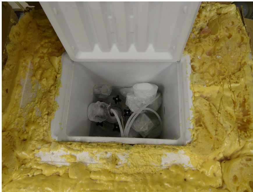
Figure 3.9: Tempe cell submerged in an ice-water
