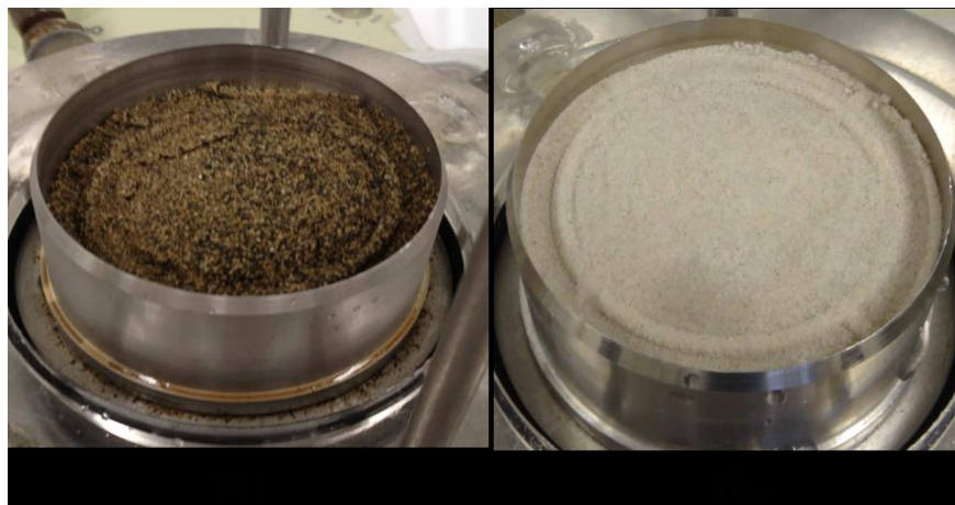
Figure B.5: Soil sample at the end of the test at temperature 49 °C (a) Industrial Sand (b)Unimin Silica Sand 7030
