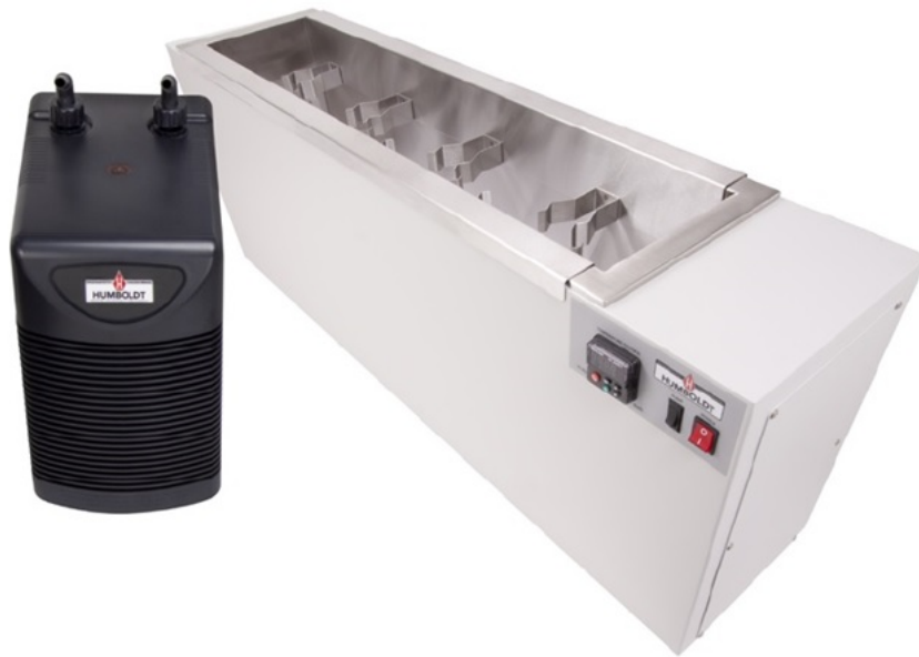
Figure B.2: Hydrometer water bath
