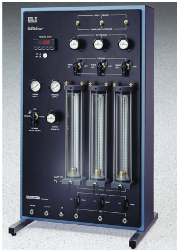
Figure B.12: Hydraulic conductivity test
