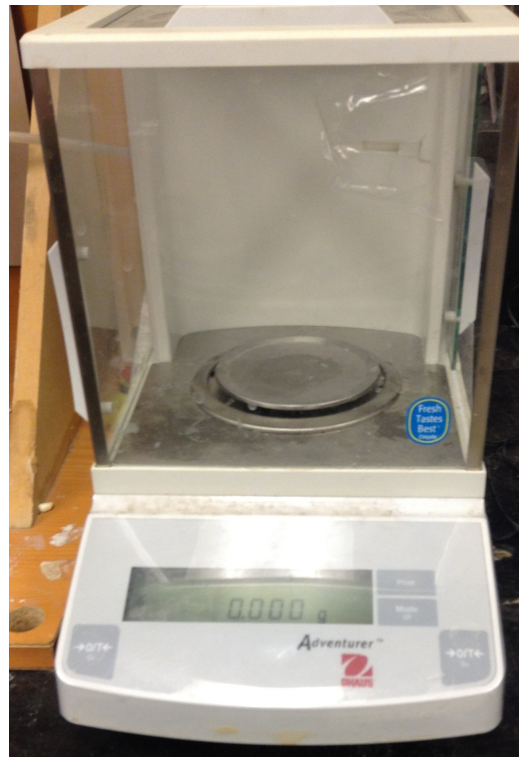
Figure B.10: Precise scale for measuring the water content of samples
