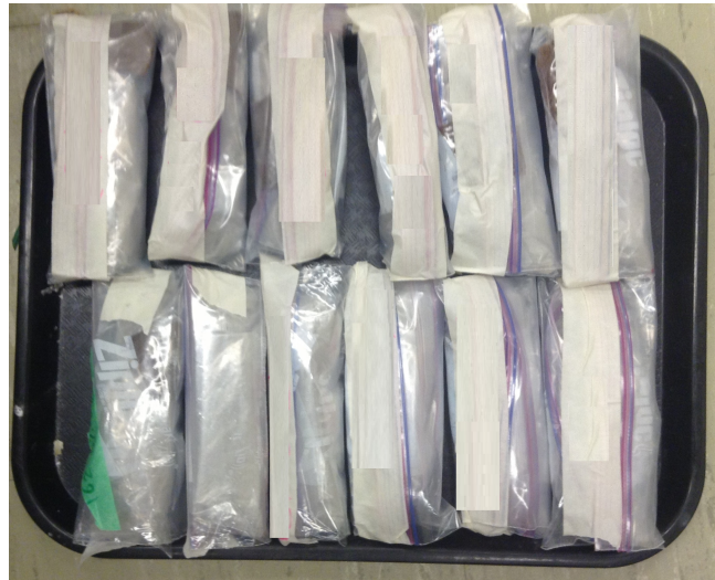
Figure B.8: Soil samples in sealed plastic bags which are stored in humidity controlled box for 2 days
