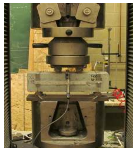
(c) Flexural beam testing machine (University of Ottawa)
