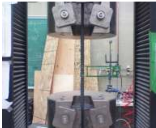
Figure 3.2 MTS testing machine
