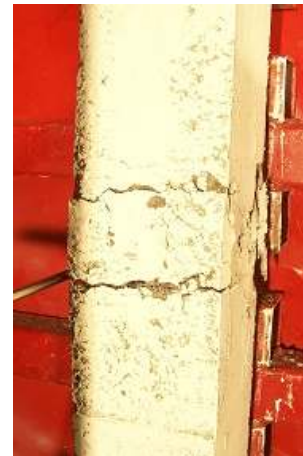
(c) Tension Face of Blast 3
