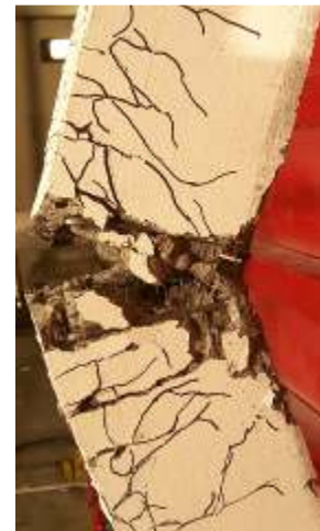
(c) Mid-Span Result of Blast 4
