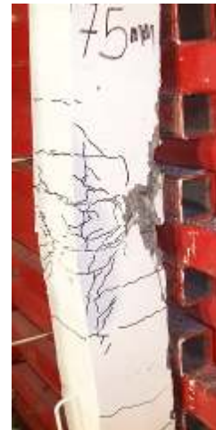
(c) Mid-Span Result of Blast 3
