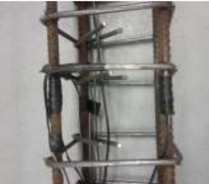
Figure 3.7 Typical cage showing strain gauge instrumentation
