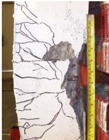
(b) Mid-Span Result of Blast 3
