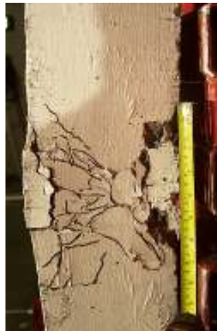
(b) Mid-Span Result of Blast 3
