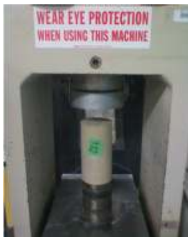
(a) Cylinder testing machine (University of Ottawa)
