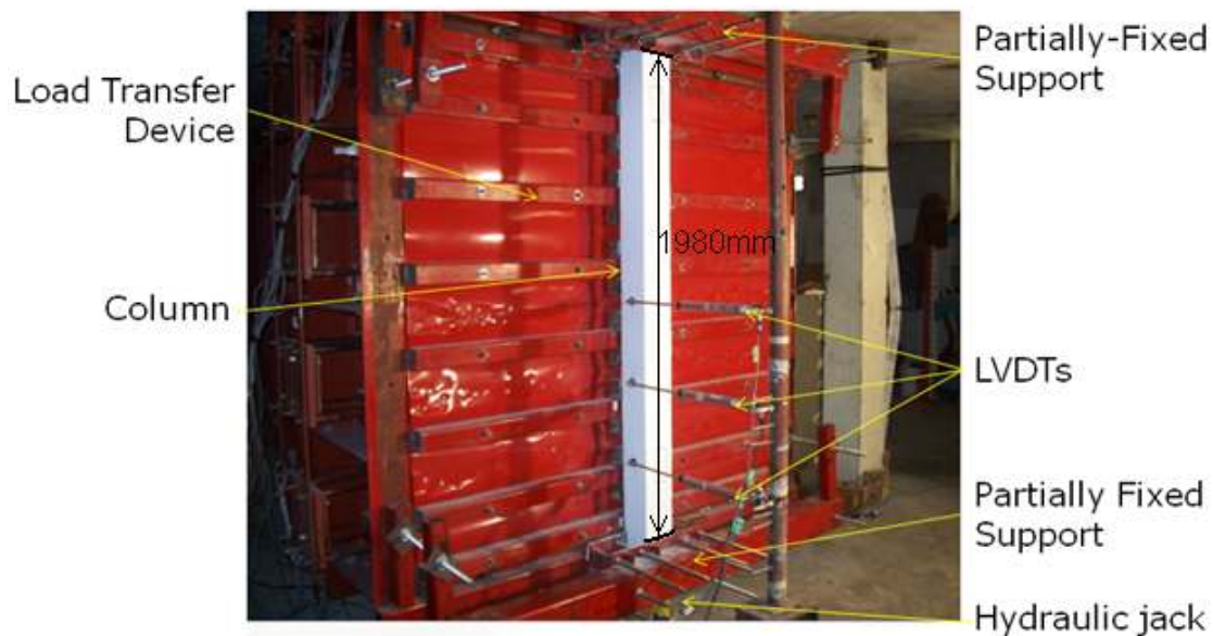
Figure 3.15 Typical test setup
