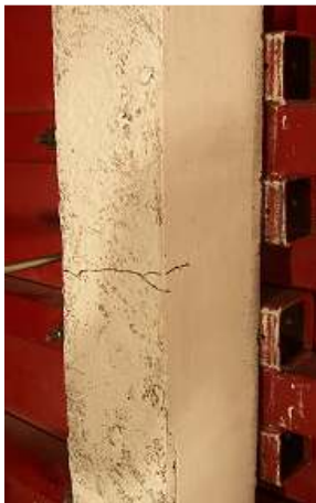
(a) Mid-Span Result of Blast 2
