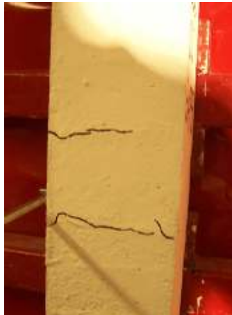
(a) Mid-Span Result of Blast 2
