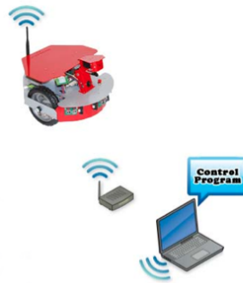
Figure 5.28: Wireless communication between the PC and X80 unit via WiFi
