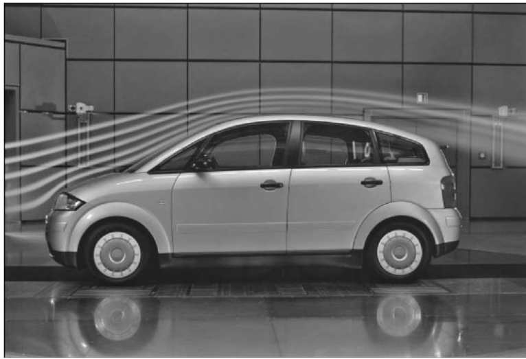
Figure 4.6: Streamlines over an automobile in a wind tunnel
