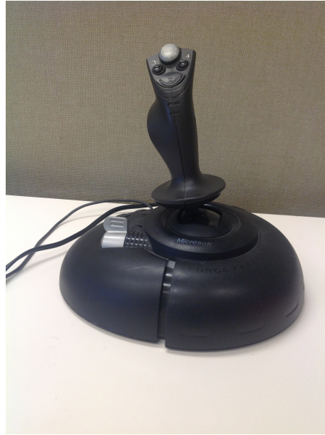
Figure 5.42: Joystick used for teleoperation with the X80
