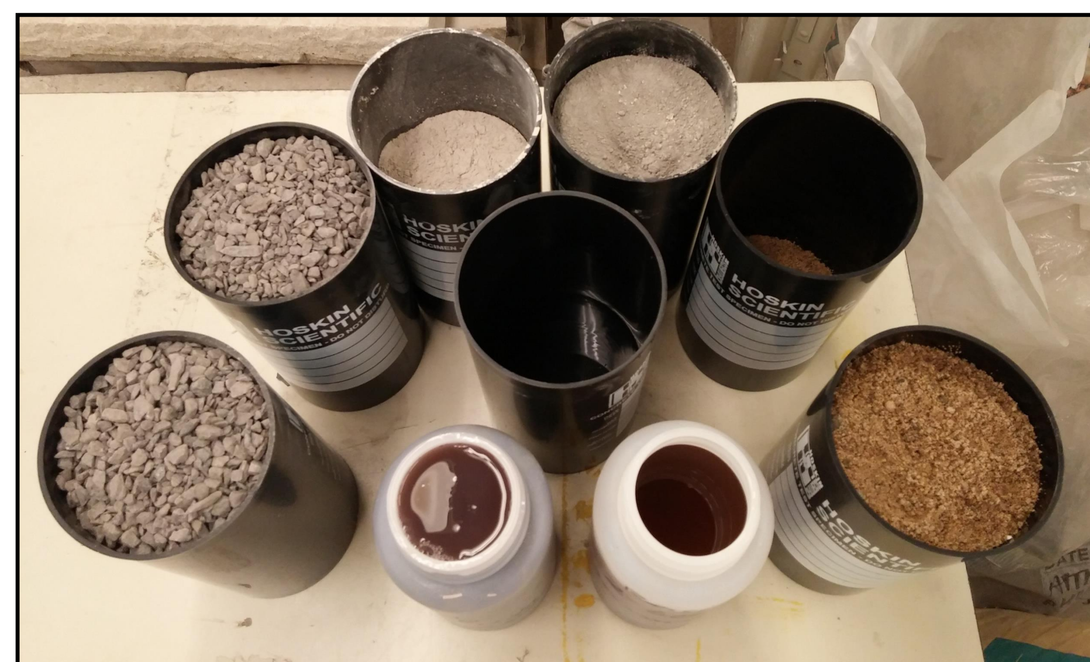
Figure #1 – Mix design materials, from left to right: Coarse aggregates, Slag / Fly Ash binder, Cement, Fine Aggregate, Water and Superplasticizer.
