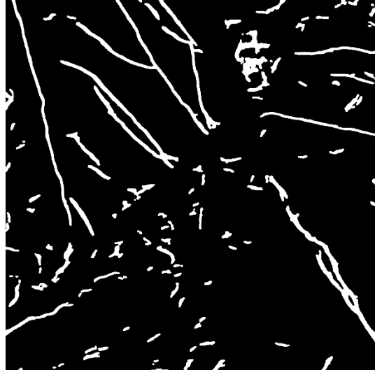
H) cracks smaller than 1mm removed
