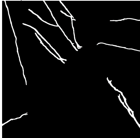
H) cracks smaller than 1mm removed
