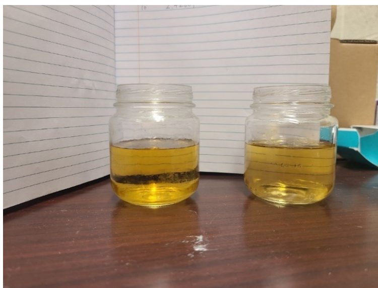
Figure 4-13. Alkaline pre-treatment supernatant after one (left) and two (right) vacuum washing cycles.
