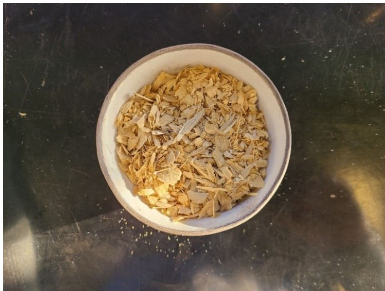
Figure 4-2. White spruce wood chips with a minimum dimension of 9.5 mm.
