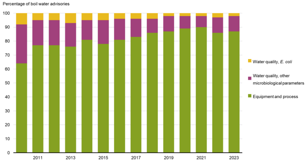
Figure 2-2. Distribution of causes of boil water advisories in Canada between 2011 and 2023 (Government of Canada, 2025b).
