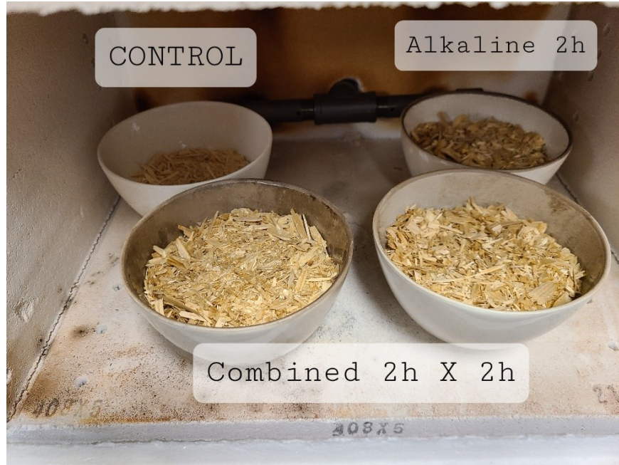
Figure 4-8. White spruce wood chips in atmosphere-controlled ashing furnace chamber.
