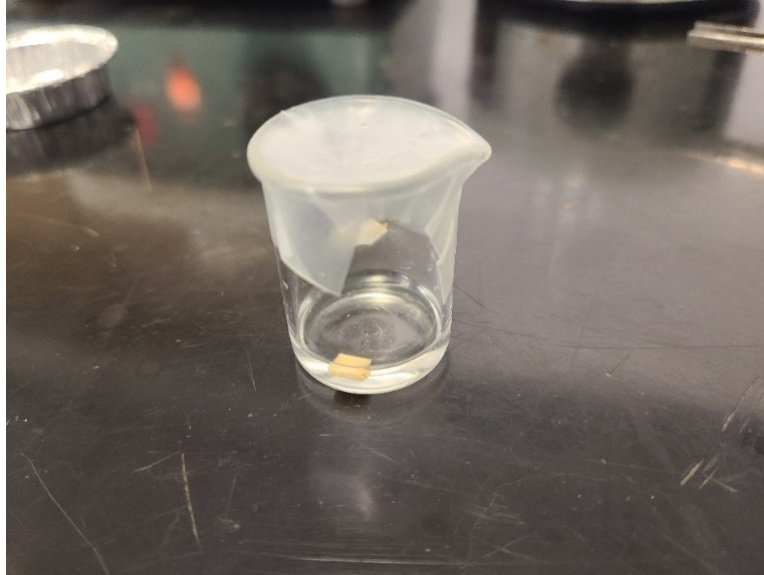
Figure 4-23. Chemical impregnation of 5 x 5 x 2 mm sample.
