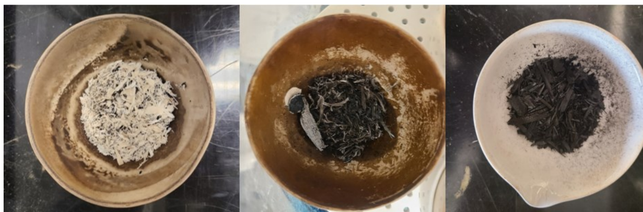
Figure 4-14. Charcoal produced from Alkaline pre-treated wood without washing (left), with vacuum washing (center), and with both vacuum and titration washing (right).
