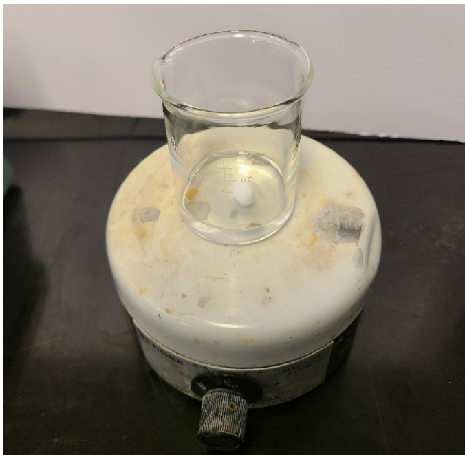
Figure 4-10. Alkaline pre-treatment apparatus for 5 x 5 x 2 mm sample.
