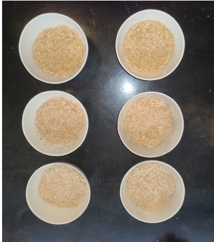
Figure 4-7. White spruce wood chips in clean, dry, ceramic crucibles.
