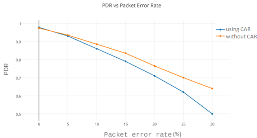
Figure 3.9: Packet Delivery Ratio vs Packet Error Rate for Big Wired Network
