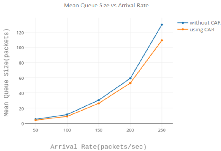
Figure 5.10: Mean Queue Size vs Arrival Rate for a Big Random Ad Hoc Network
