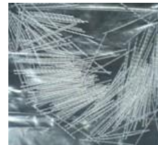
Figure 3.1 Shape of fibers used in this project a) Steel fibers b) Polypropylene fibers
