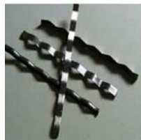
Figure 3.1 Shape of fibers used in this project a) Steel fibers b) Polypropylene fibers
