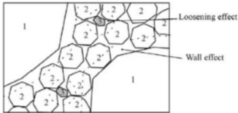
Figure 2.2 Wall Effect and Loosening Effect
