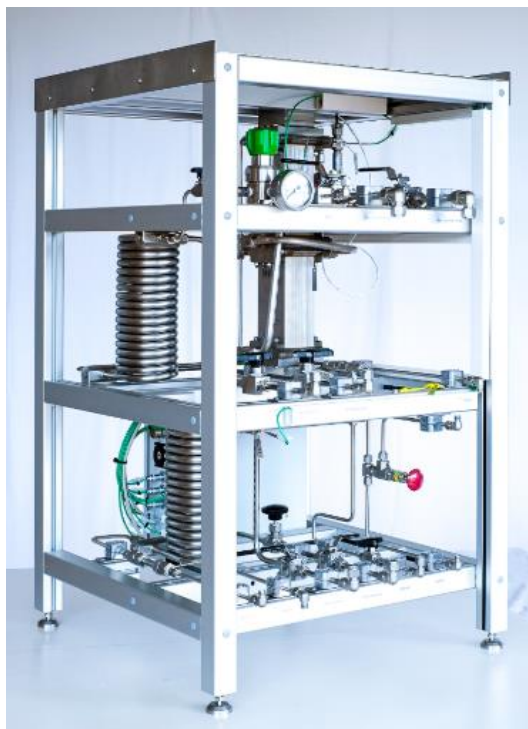
Figure 2.8. Reactor platform module. Reprinted with permission from reference [88]. Copyright 2015 Microinnova.
