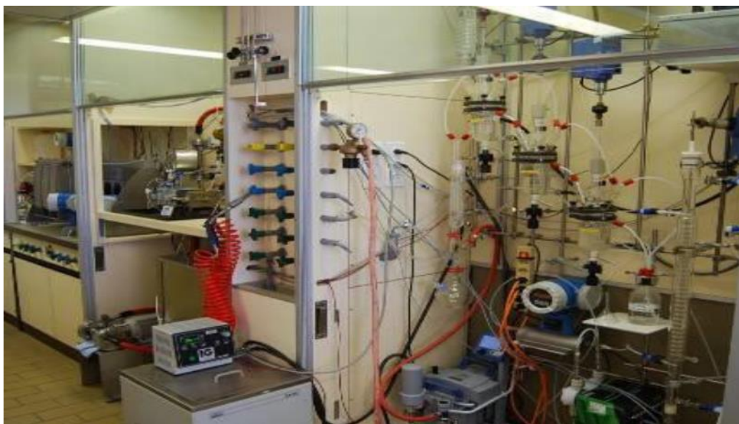
Figure 2.5. Lab-based development of a continuous mini-monoplant contained within three fume hoods.
