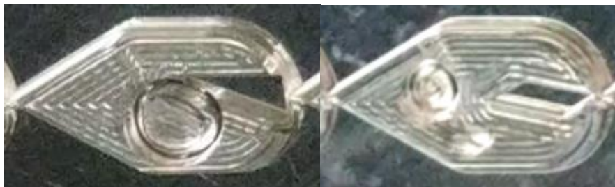
Figure 3.5. Flow in LL-Triangle (left) demonstrating increased gas holdup in centre of mixer, a behaviour that is absent in the LL-Rhombus (right) for the same flow rates. Liquid velocity is 0.53 m/s, and gas velocity is 0.080 m/s in the LL-Triangle and 0.081 m/s in the LL-Rhombus.
