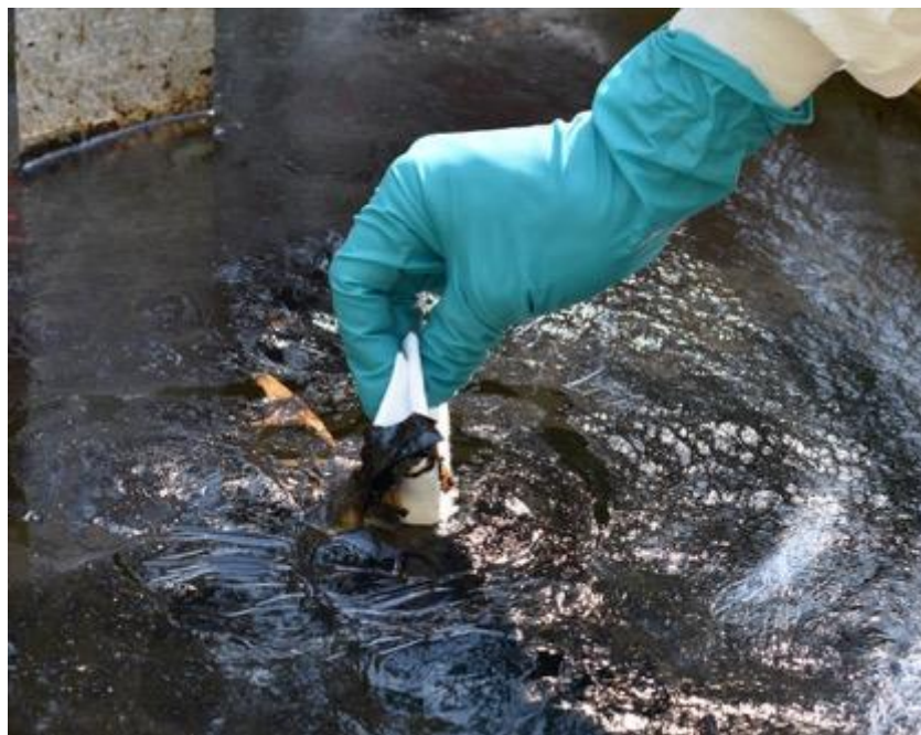
Figure S2. 3. Surface slick sample collected from the high-treatment microcosm utilizing a section of polyester absorbent pad
