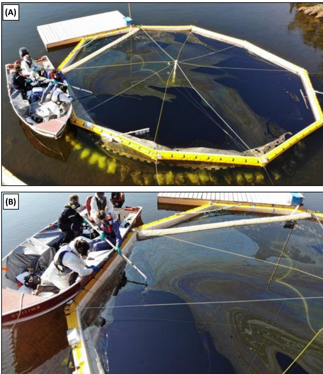
Figure S3. 1. The addition of 180 L of CLWB (1:590 oil:water, v/v) onto the water surface of the limnocorral. (A) Overview of addition method, (B) View of telescopic arm and pumping system being held at approximately 5 – 10 cm from the water's surface. The oil exited the hose parallel to the water's surface to avoid forcing oil below the water surface and allowing it to spread out during the addition.
