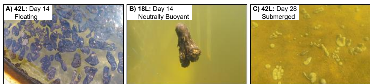
Figure S3. 3. Examples of tar balls observed floating on the water surface (A), neutrally buoyant in the water column (B), and submerged on the sediments (C).
