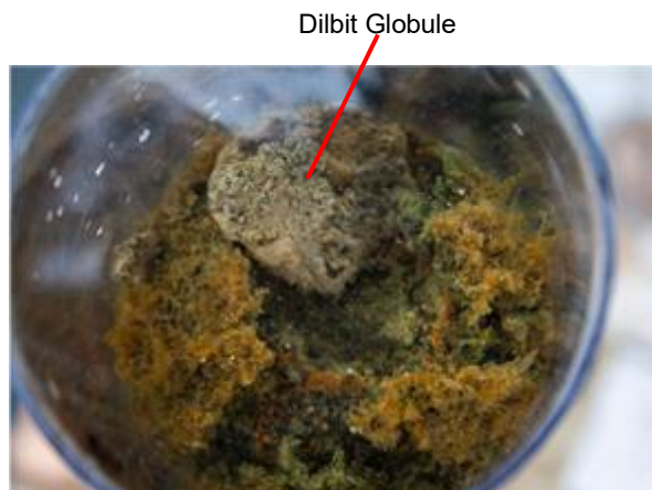
Figure S5. 4. Example of a tarball sitting on top of the sediment in a coring tube. The tarball was removed and then the top 1cm of the core was processed for PAH analysis.
