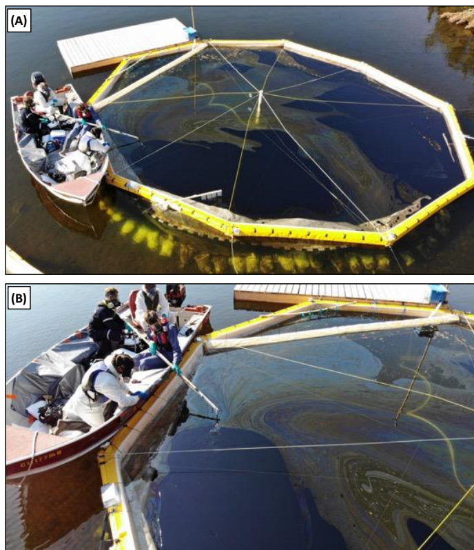
Figure S5. 1. Schematic of limnocorral set up showing water and sediment sampling methods.
